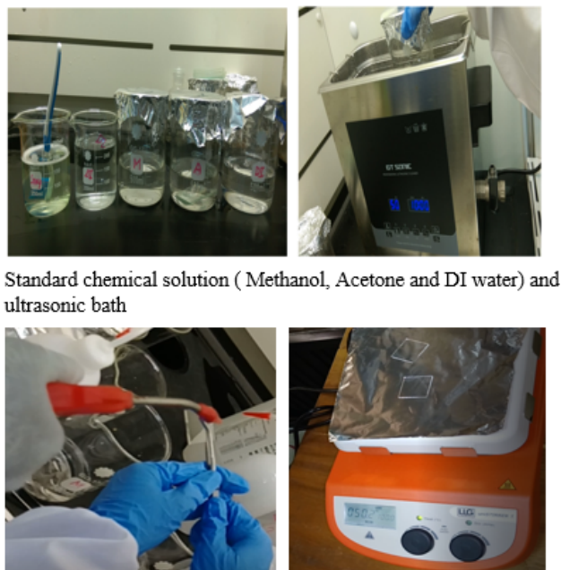
Drying of SLG substrate through nitrogen gas and on Hot plate.
