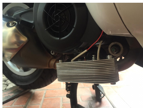
Fig. 12. Location of harvester unit installation.
