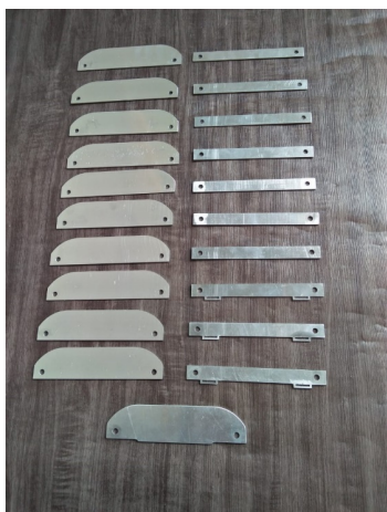
Fig. 9. Heat sink part assembly.
