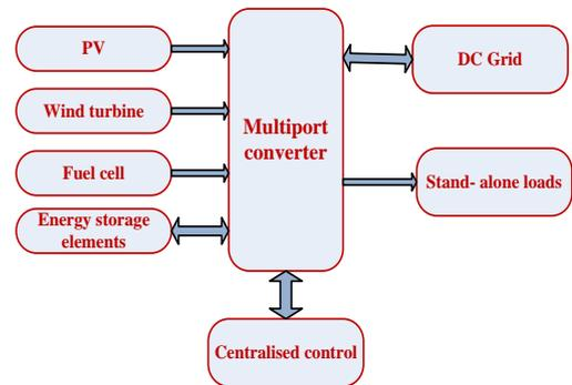
Fig. 1 Multiport converter-Schematic
