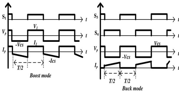
Fig. 8 Key waveforms of Three- port partially isolated bidirectional converter
