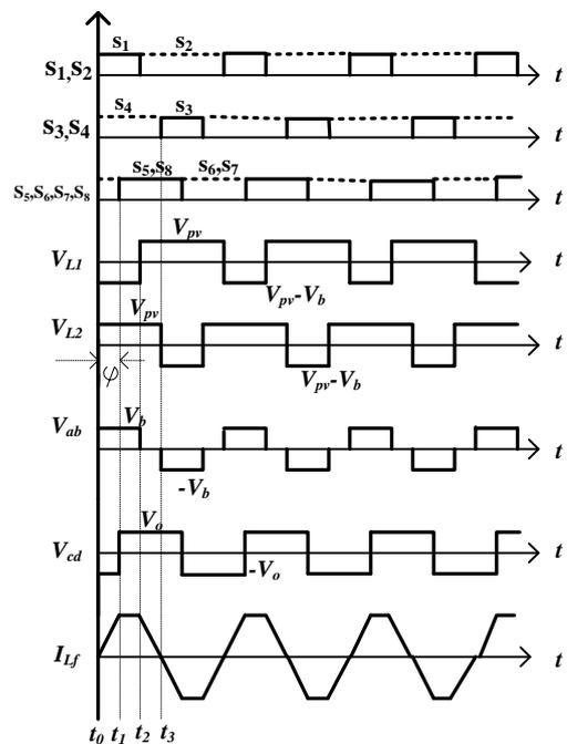
**Fig. 16** Key waveforms of Full bridge three port bidirectional converter
