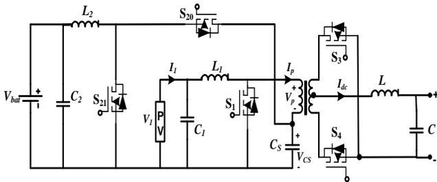
Fig. 7 Bidirectional partially isolated three-port dc-dc converter
