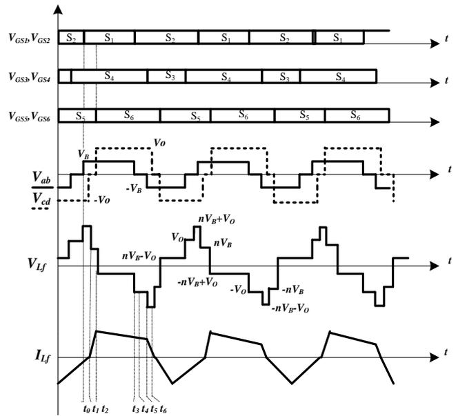
Fig. 12 Key waveforms of PWM and secondary side phase shifted converter
