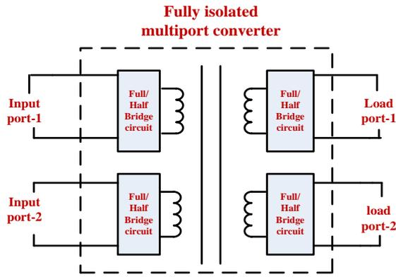
Fig. 3 Fully-isolated multiport topology
