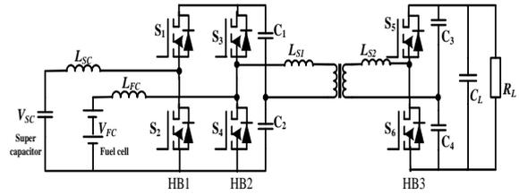
Fig. 5 Multi-input bidirectional dc-dc converter
