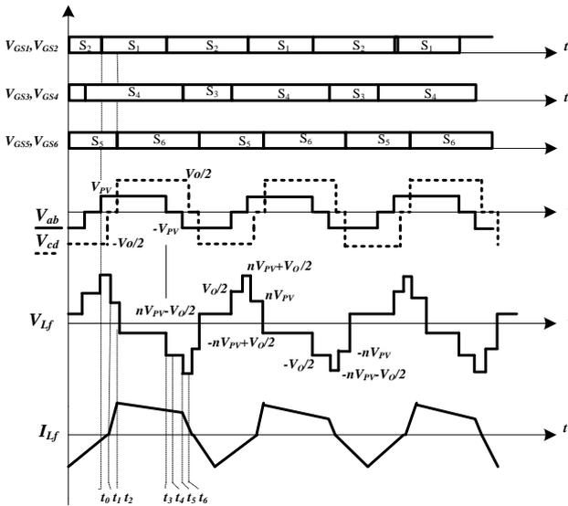
**Fig. 14.** Key waveforms of secondary side regulated converter
