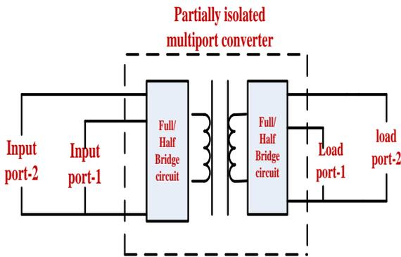
Fig. 4 Partially- isolated multiport topology
