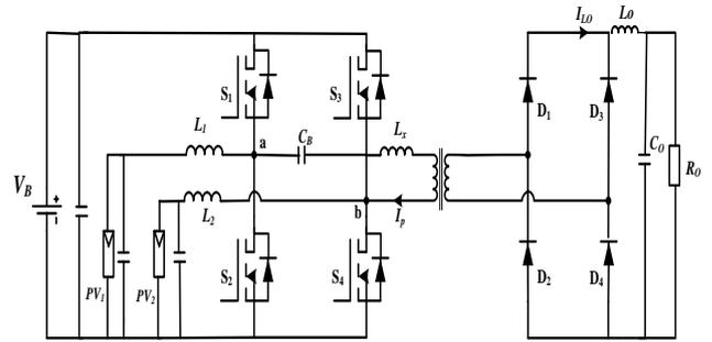
Fig. 9 Buck-Boost four port converter
