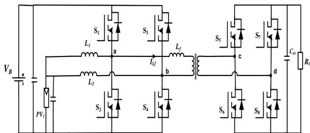
**Fig. 15** Full bridge three port bidirectional converter
