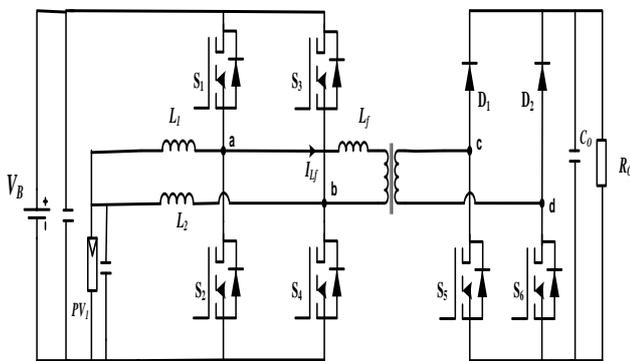
Fig. 11 PWM and secondary side phase shifted converter
