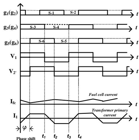
Fig. 6 Key waveforms of the multi-input bidirectional converter
