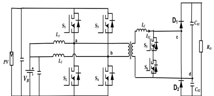
Fig. 13 Secondary side regulated converter
