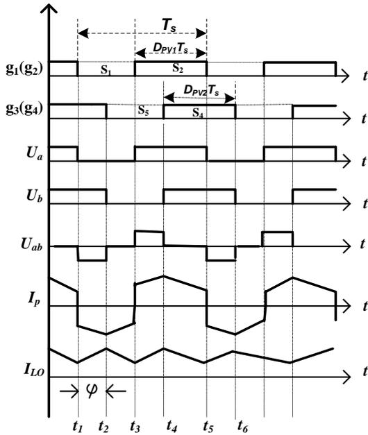
Fig. 10 Key waveforms of Buck-Boost four port converter
