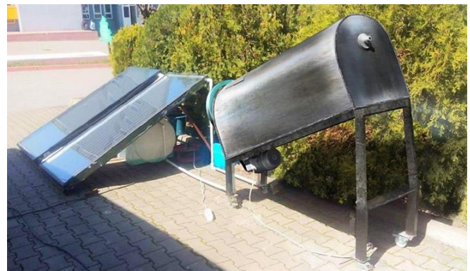
Fig. 1. View of the drying chamber and solar energy production unit
