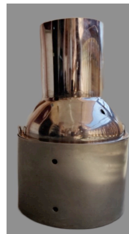
Fig. 7. Stainless steel chamber used for conducting the experiment
