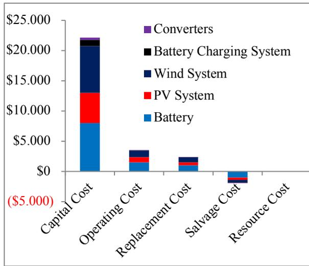
Fig. 14. Annualized cash flow summary by hybrid system component PV-wind-battery-converter
