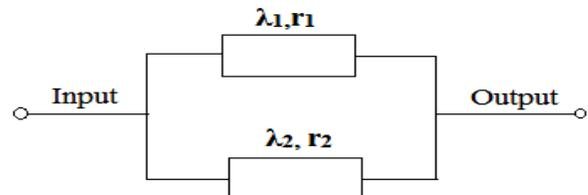
Fig.9. Parallel components system
