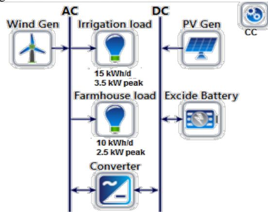
Fig. 12. HOMER simulation model of hybrid PV-Wind-battery energy system
