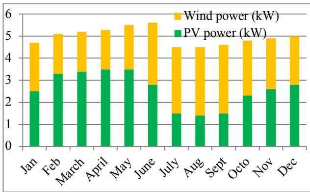
Fig. 15. Monthly average electric production of PV and wind generator
