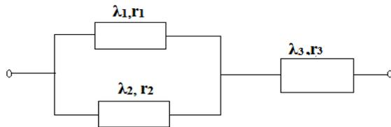
Fig. 10 Series-parallel configuration
