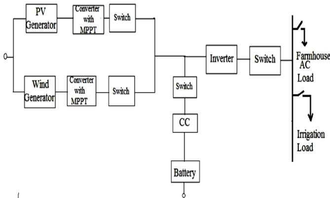
Fig. 5. Reliability block diagram of hybrid energy system
