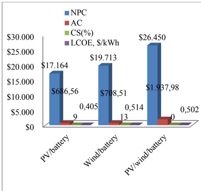
Fig.13 Comparison of NPC, AC, LCOE and capacity shortage of different configurations
