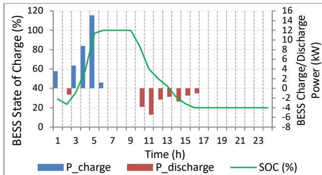
Figure 20. BESS charge/discharge power and SOC (Case 4)
