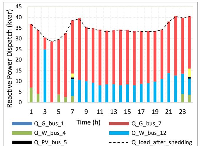
Figure 18. Reactive Power Dispatch from the Different Sources (Case 4)
