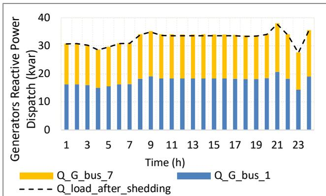
Figure 15. Reactive Power Dispatch of Diesel Generators (Case 3)
