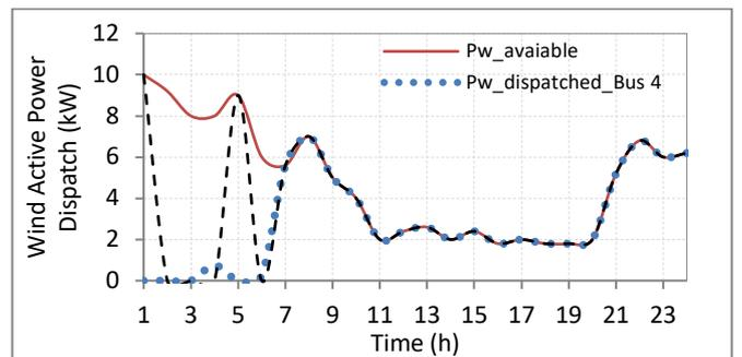
Figure 19. Dispatched wind and its curtailment (Case 4)
