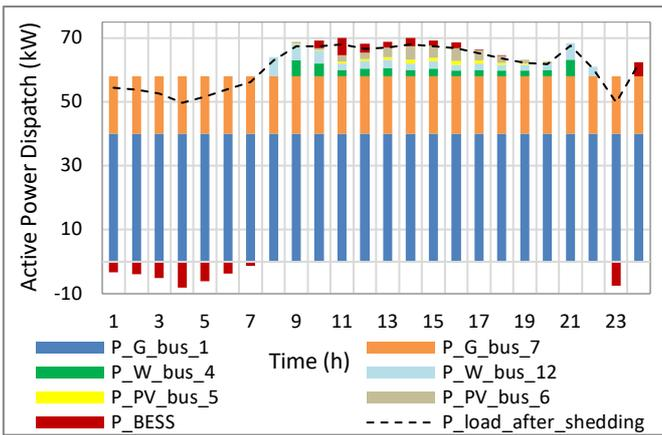
Figure 14. Active Power Dispatch from the Different Sources (Case 3)
