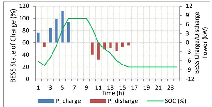
Figure 11. BESS charge/discharge power and SOC (Case 2)
