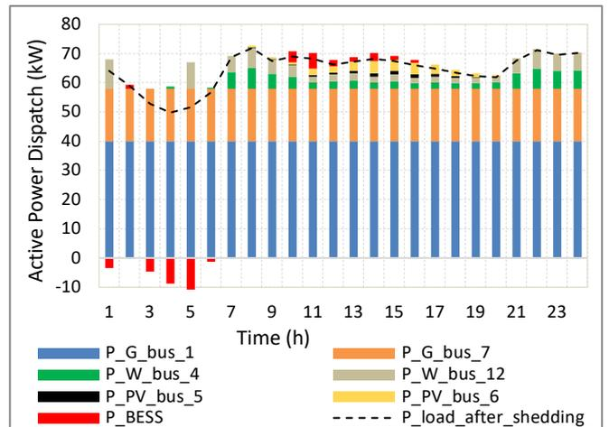
Figure 17. Active Power Dispatch from the Different Sources (Case 4)
