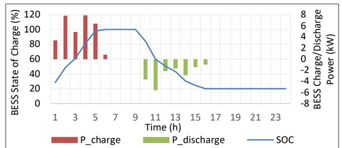
Figure 7. BESS charge/discharge power and SOC (Case 1)
