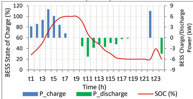
Figure 16. BESS charge/discharge power and SOC (Case 3)
