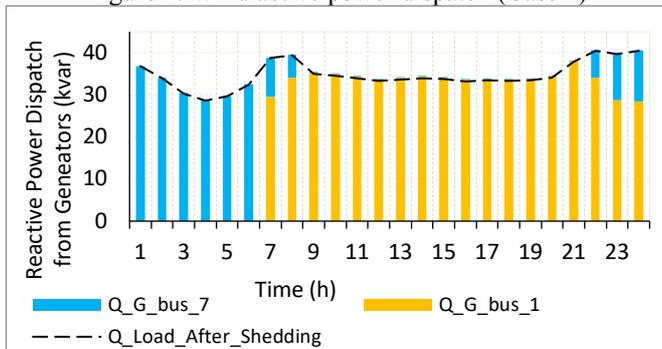
Figure 5. Reactive Power Dispatch of Diesel Generators (Case 1)
