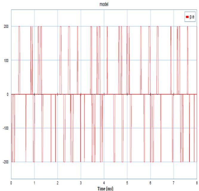
Fig. 7. Voltage signal measured at the inverter output (20-Sim simulation).
