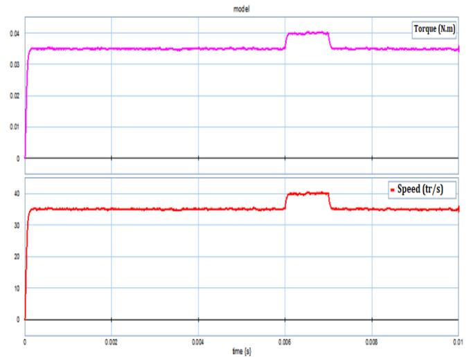
**Fig. 16.** Measurements at the motor side with a hydraulic fault: (a) torque, (b) Angular Speed
