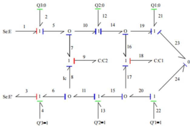
Fig. 6. Corresponding BG model of the 3 phased inverter.
