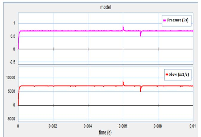
**Fig. 17.** Measurements at the Pump side with hydraulic fault: (a) Pressure, (b) Flow rate
