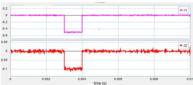
**Fig. 15.** Residues r1 and r2 with a sudden mechanical fault
