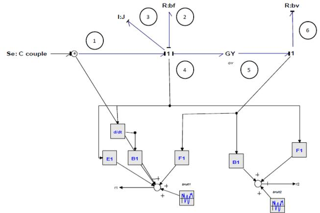
Fig. 11. Complete 20-Sim simulation model (BG model + Diagnosis system).
