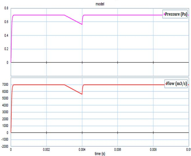
**Fig. 14.** Measurements at the Pump side with mechanical fault: (a) Pressure, (b) Flow rate
