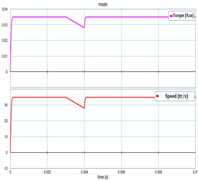
**Fig. 13.** Measurements at the motor side with a mechanical fault: (a) torque, (b) Angular Speed
