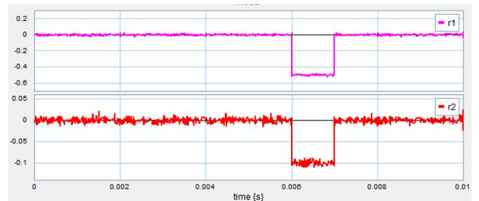
**Fig. 18.** Residues r1 and r2 with a sudden hydraulic fault
