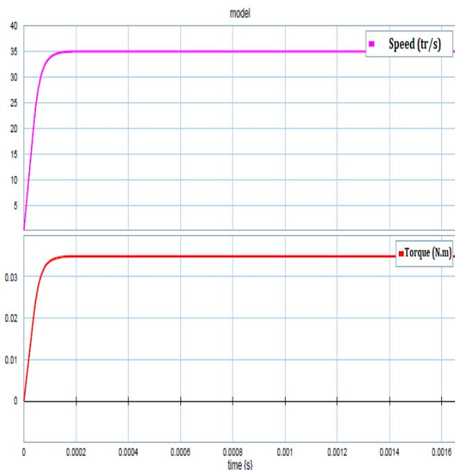
Fig. 9. Motor measurements of the developed BG model: (a) Angular speed, (b) torque
