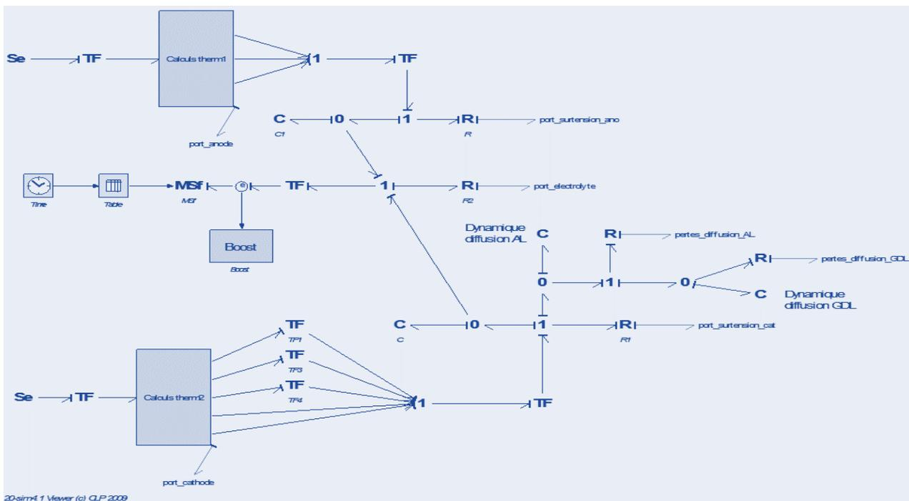
Fig. 4. Detailed BD modeling of the PEMFC+Boost converter.
