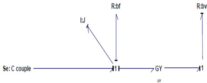
Fig. 8. Moto pump Bond Graph model
