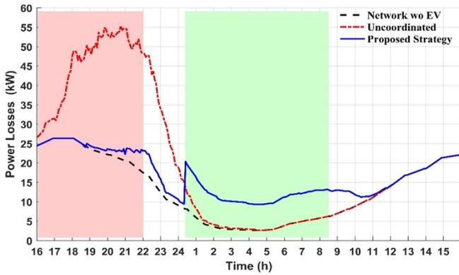
Fig. 12. Network overall power loss.
