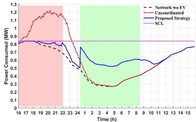
**Fig. 11.** Total network power consumption at the substation.
