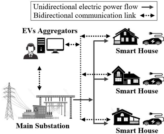
Fig. 4. Schematic diagram of the centralized coordinated charging.
