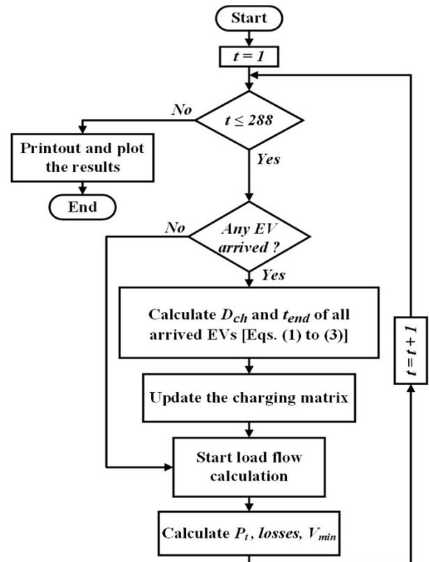
Fig. 3. Main procedures of the uncoordinated charging mode.
