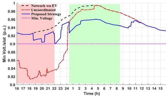
Fig. 13. Network minimum voltage magnitude.
