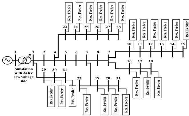
Fig. 8. Modified IEEE 31 bus distribution network.
