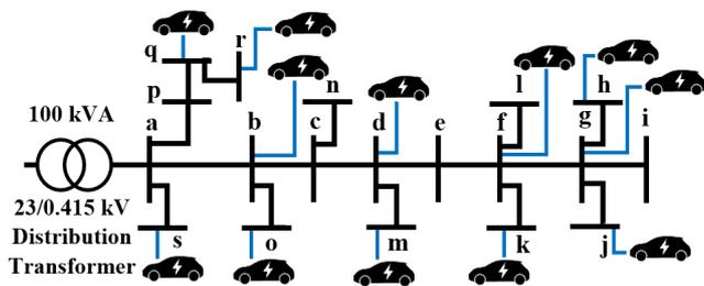
Fig. 9. Residential feeder with 63% EV penetration level.
