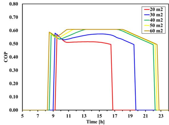
Fig. 7. Variation of the adsorption chiller COP for the PTC collector at different collector areas.
