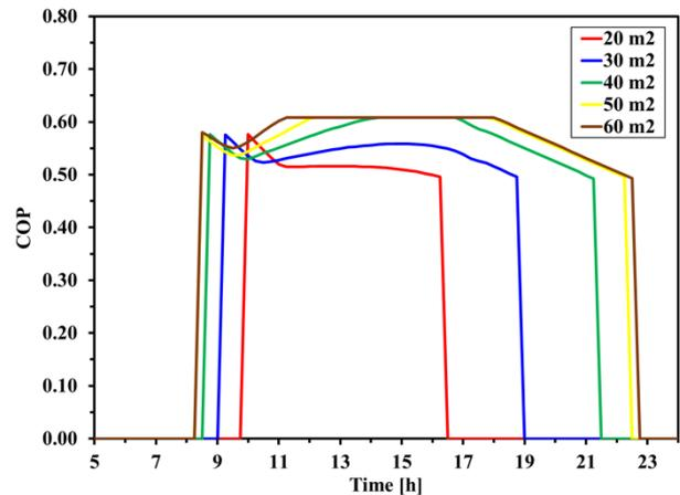
Fig. 8. Variation of the adsorption chiller COP for the CPC at different collector's areas.
