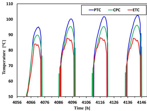
Fig. 5. Comparison between the outlet temperature for the PTC, CPC, and ETC solar collectors.
