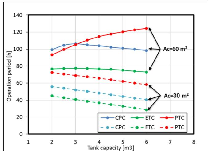
Fig. 12. Effect of the storage tank capacity on the weekly operation period of the adsorption chiller for PTC, CPC, and ETC for two collector's surface areas.
