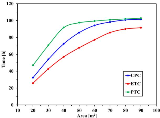
Fig. 11. Variation of the weekly chiller operation period of the PTC, CPC, and ETC at a storage capacity of 2.55 m<sup>3</sup>.
