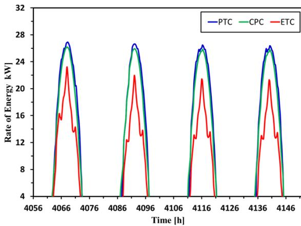
Fig. 6. Comparison between the rate of collector energy gained for the PTC, CPC, and ETC.
