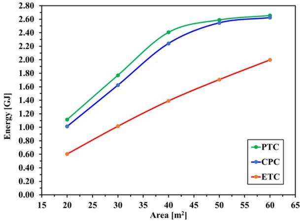
Fig. 10. Variation of the weekly chiller cooling energy of the PTC, CPC, and ETC at a storage capacity of 2.5 m<sup>3</sup>.
