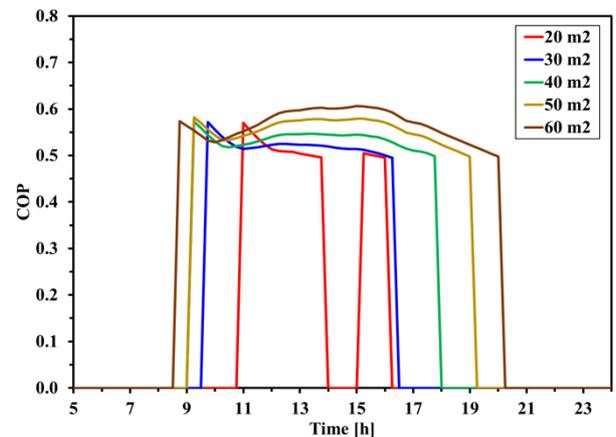
Fig. 9. Variation of the adsorption chiller COP for the ETC collector at different collector areas
