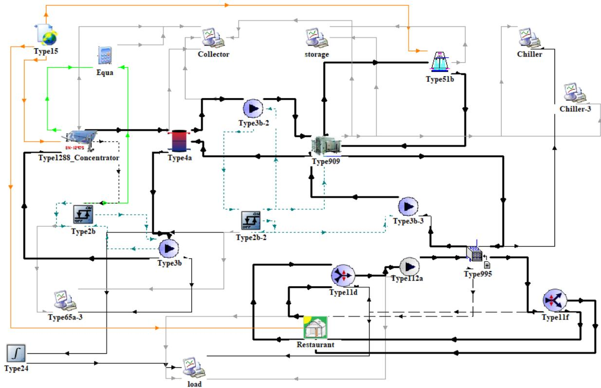
Fig. 2. View of the TRNSYS project for the solar adsorption cooling system.
