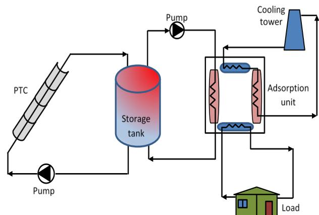
Fig. 1. Schematic diagram of the solar adsorption refrigeration system
