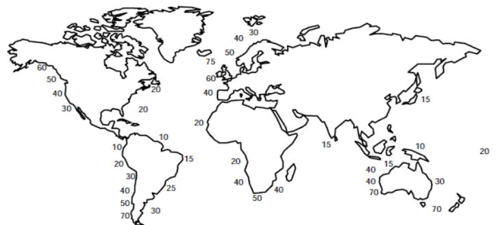
**Figure 1:** World wave power estimation in kW/m
