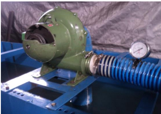
Fig. 9. A pressure gauge is installed at the end of the inlet pipe
