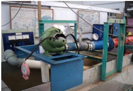
Fig. 5. BAT installed in the test installation
