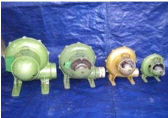
Fig. 1. Centrifugal blowers of size 4-inch, 3-inch, 2.5-inch, and 2-inch not modified ( \beta < 90^\circ )
