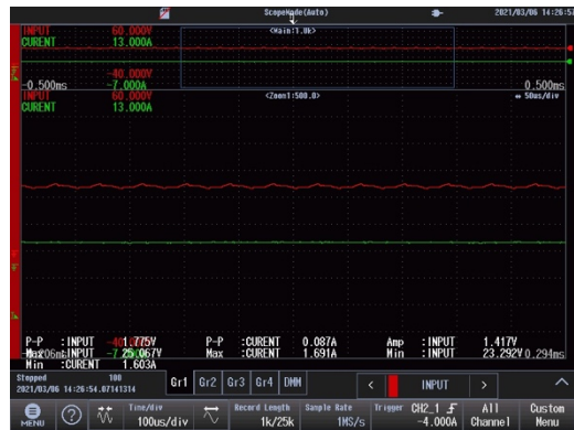
Fig 29. Output voltage and currents of the two phase interleaved converter in buck mode
