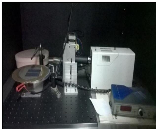
Fig. 2. SPV measurement system.
