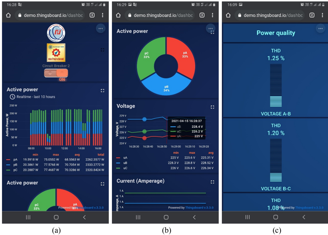
Fig. 9. The monitoring and controlling screen on the smartphone of the Node station: (a) Active power monitoring, (b) Voltage and current monitoring, (c) Total harmonic distortion monitoring.
