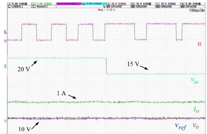
Fig. 23. Experimental responses of the output voltage and the CPL current for the step-change in v_{in} from 20 V to 15 V
