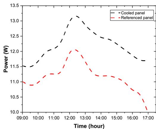
Fig. 8 Power variation for the two modules
