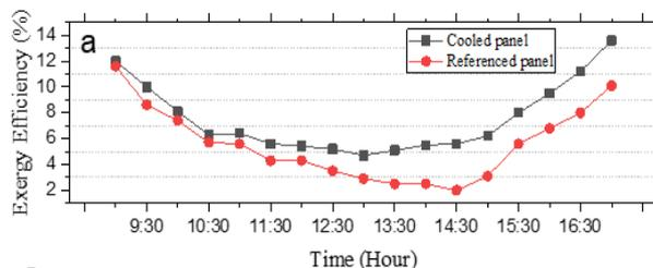
Fig. 10 (a) Exergy efficiency (b) thermal efficiency for both panels
