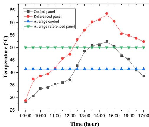
**Fig. 4.** Temperature characteristics of the two panels
