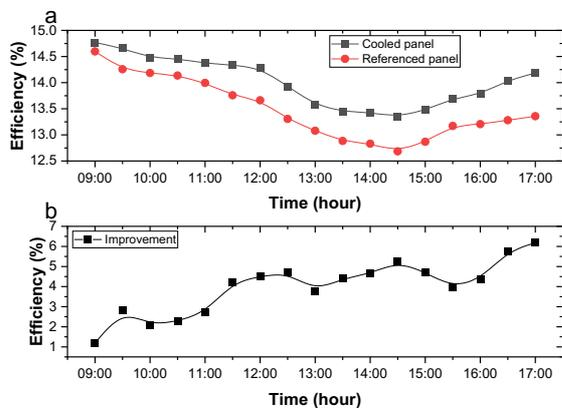
Fig. 9 Efficiency variations and improvement for the panels
