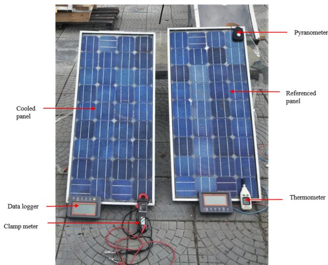
**Fig. 2** Experimental test rig - cooled or modified panel (left) referenced panel (right)
