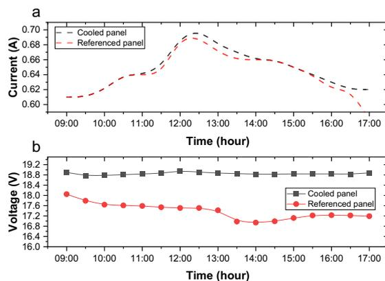
**Fig. 7** (a) Current and (b) voltage variations for the two panels
