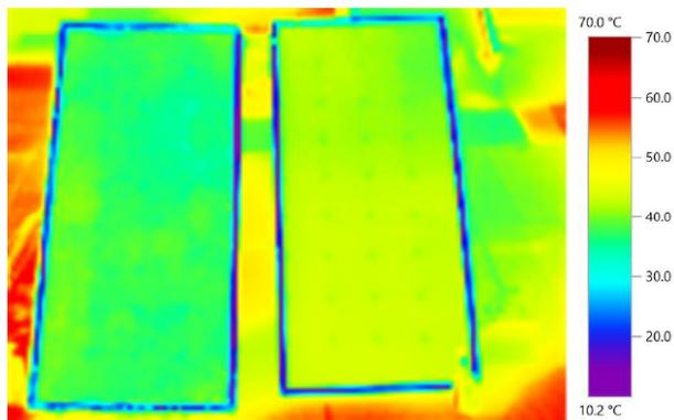
**Fig. 5** Thermal image of the two panels - cooled (left) referenced (right)
