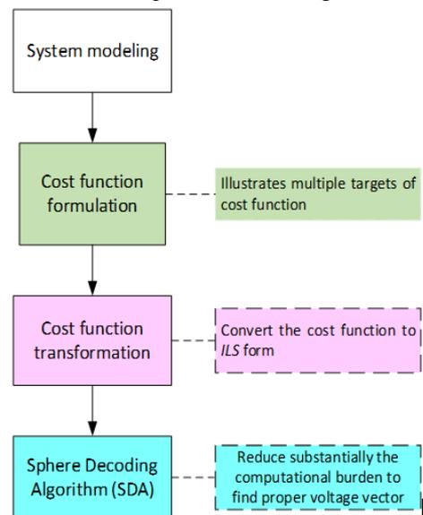
Fig. 2. Multi-step MPC for current controller
