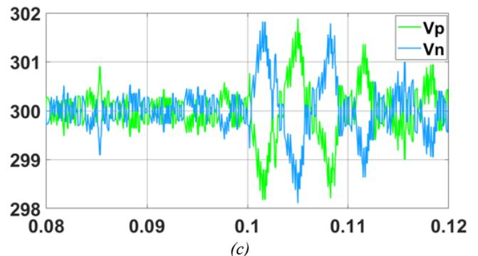
**Fig. 6.** Voltage balance on 2 input DC capacitors
