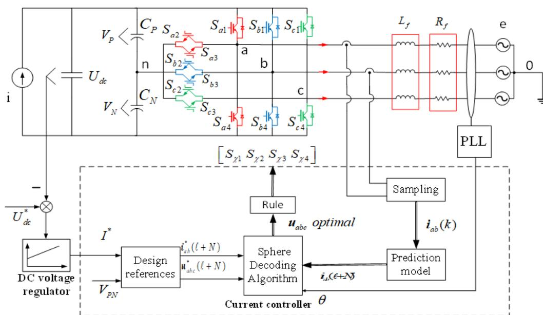
Fig. 1. Control structure for three-phase T-Type inverter in grid-connected mode using Multi-step MPC strategy
