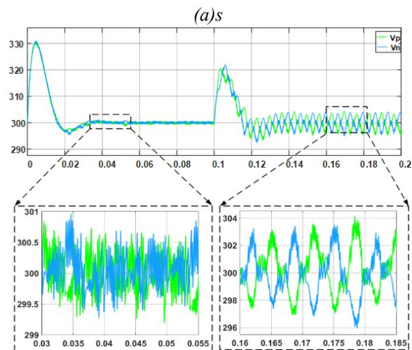
Fig. 11. Voltage balance on 2 input capacitors
