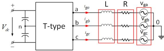
**Fig. 3.** Grid- connected model with L filter
