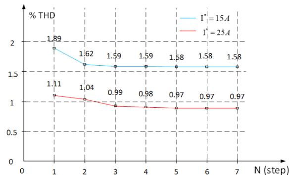
**Fig. 8.** THD of the grid-connected current vs the number of prediction steps
