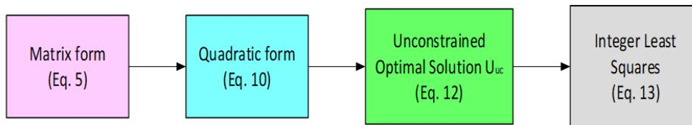
**Fig. 4.** Four steps to transform the cost function
