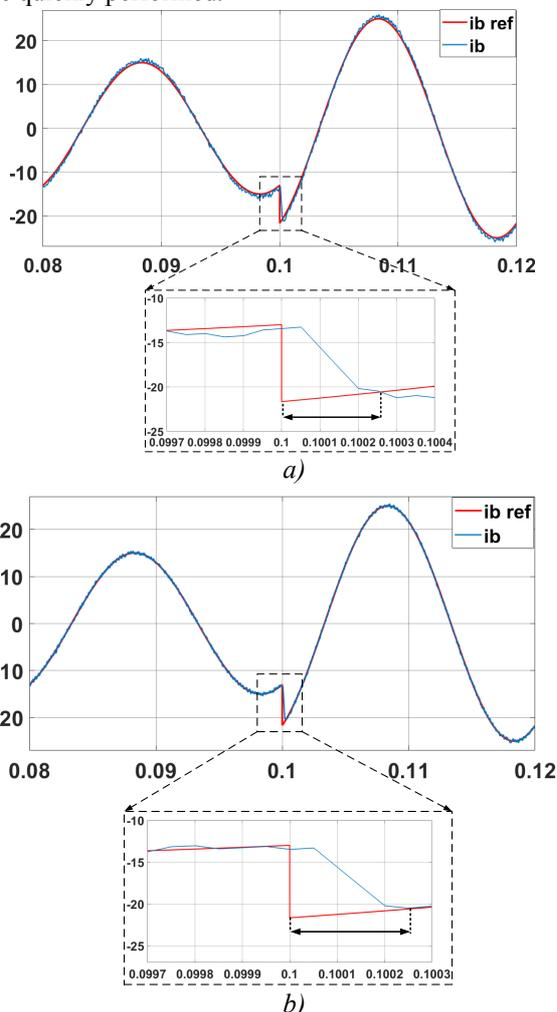
Fig. 10. Dynamic performance of the grid-connected current
