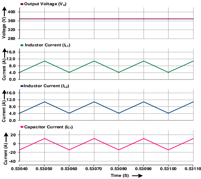
Fig. 8 Simulation results of output voltage and passive elements current
