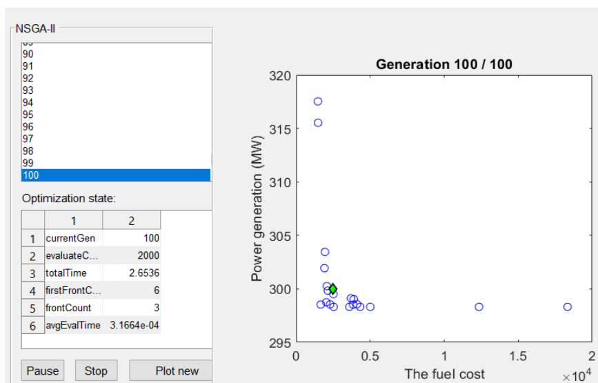
Fig. 5. The solutions of all generations including Pareto optimal solutions based on RNSGA- II with losses
