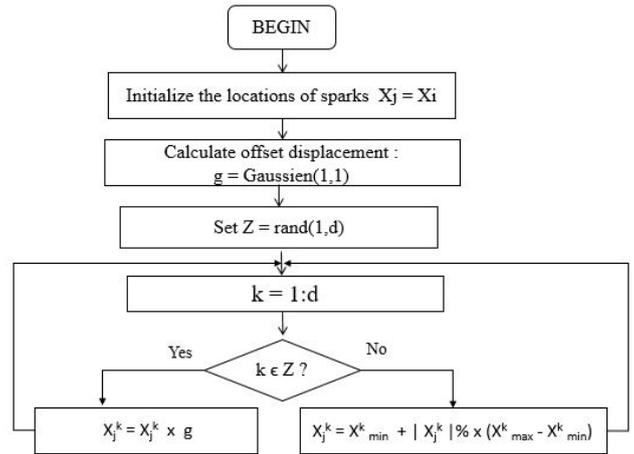
Fig. 5. Flowchart of mutation operator.
