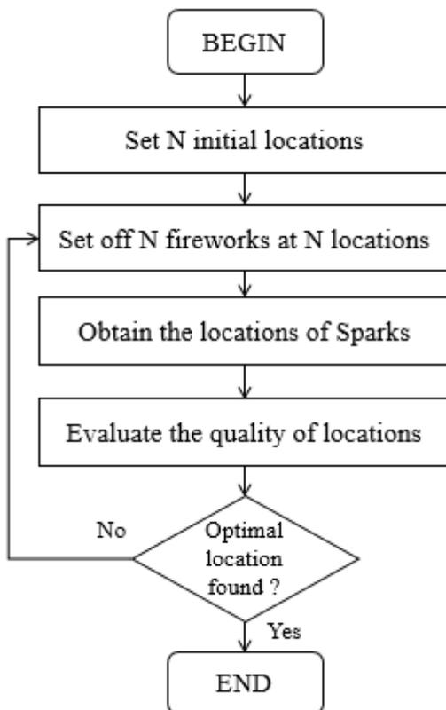
Fig. 2. Flowchart of FWA algorithm.
