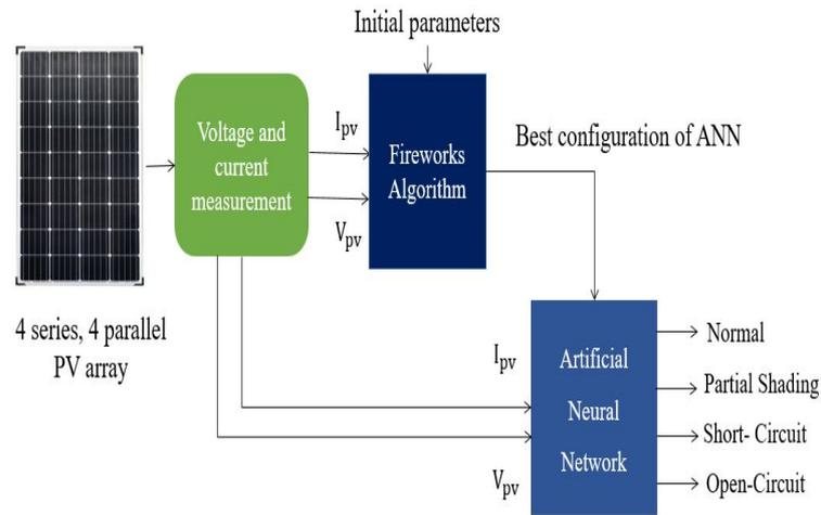
Fig.7. Schematic diagram of FWA-ANN model for diagnosing PV Field.
