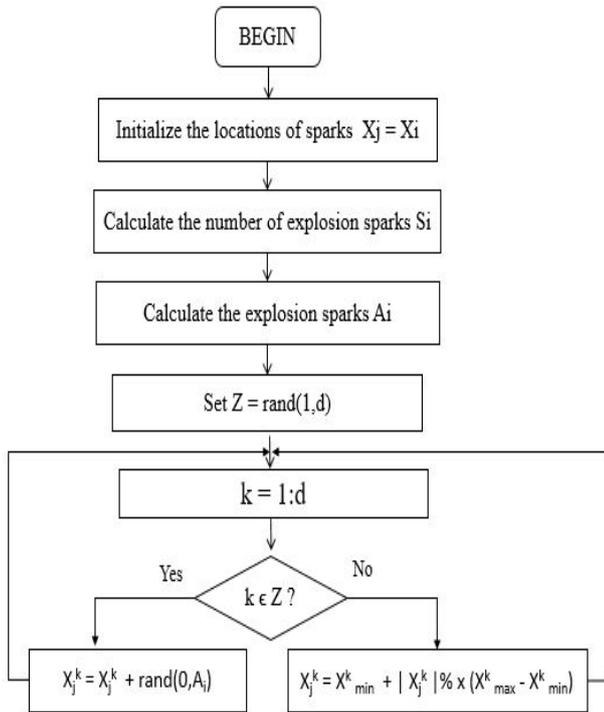
Fig.4. Flowchart of explosion operator.
