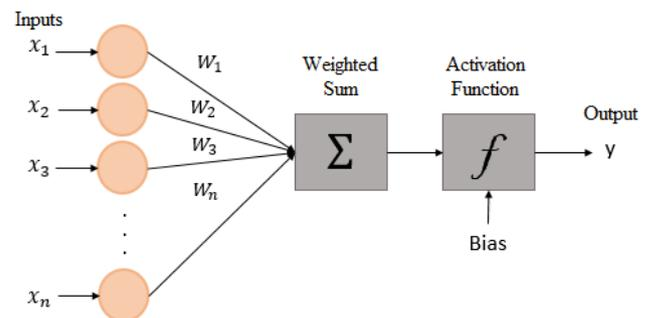
**Fig. 1.** Representation of an artificial neuron.
