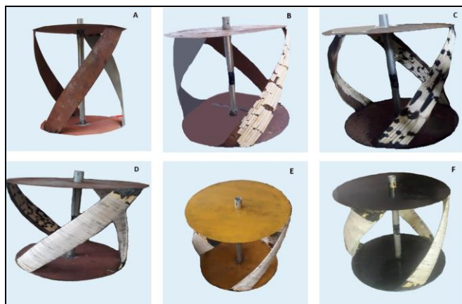
Fig. 12. Various stages of manufacturing GHT
