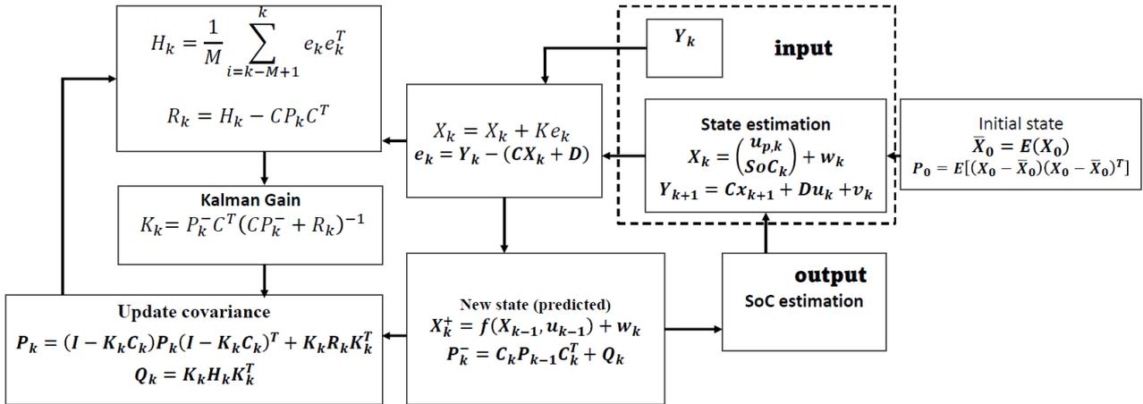
Fig. 3. Schematic scheme for AEKF algorithm
