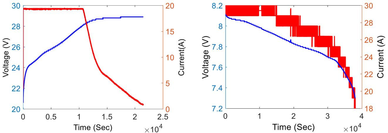
**Fig. 5.** Current and voltage; (a) charging and (b) discharging profile
