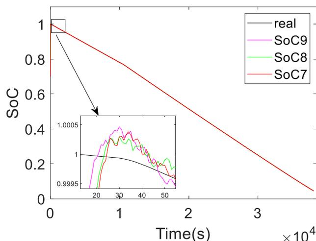
**Fig. 9.** SOC Estimation Based on Different Initial of SOC
