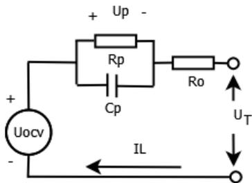
**Fig. 2.** Electrical Equivalent Circuit Model Lithium-Ion Battery
