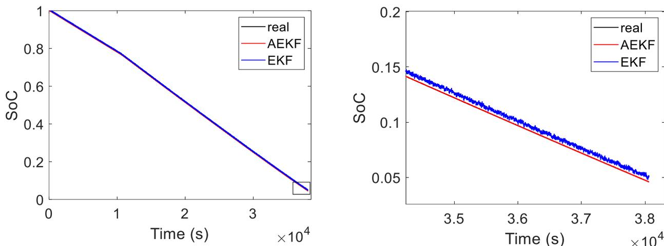
**Fig. 8.** SoC Estimation result with noise (a) SoC Estimation; (b) Details
