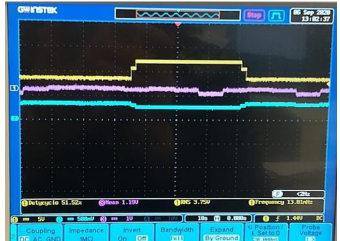
Figure 23. Case 4; PV ON, battery status changing when load power changing.
