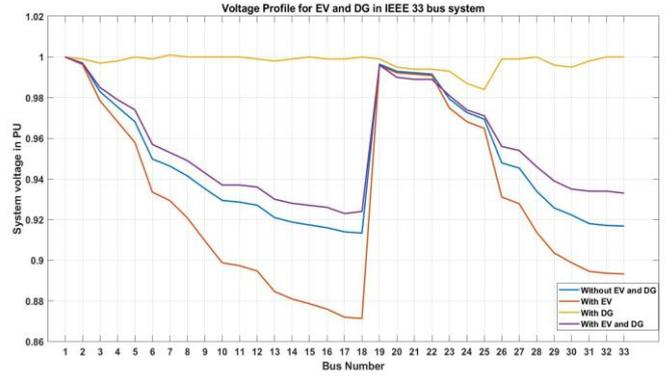
**Fig.8.** Voltage levels in IEEE 33 Bus system with possible cases.
