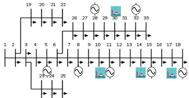
**Fig.6.** Optimal placement of EVs and DGs for an IEEE 33 bus system.
