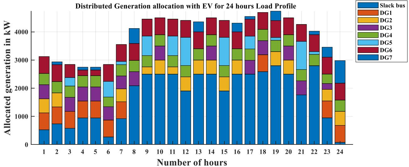
**Fig.11.** Optimal scheduling of DGs for 24-hour load profile using AOA
