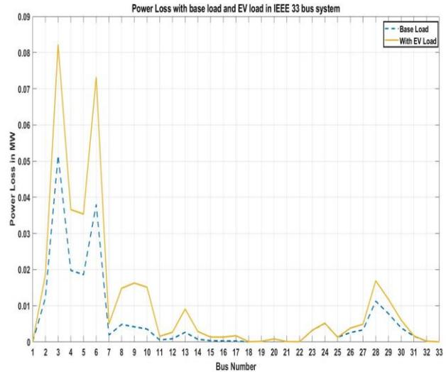
Fig.1. Power Loss of IEEE 33 bus system with EV Load.
