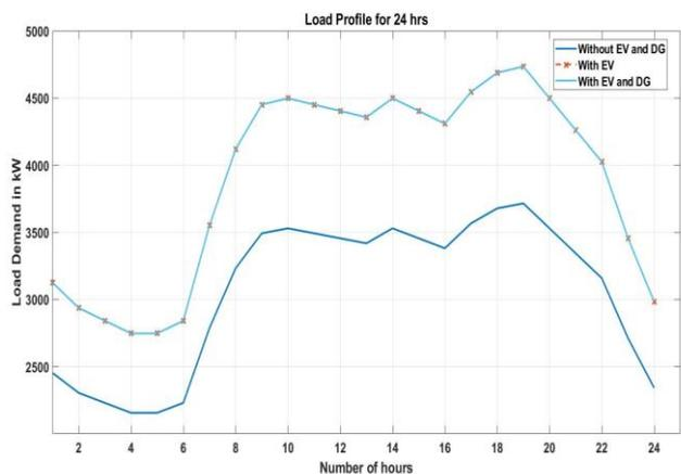
Fig.9. Load profile for 24-hour load setting with possible cases.
