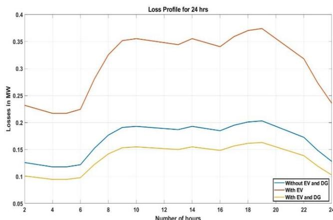
Fig.10. Loss profile for 24-hour load setting with possible cases.
