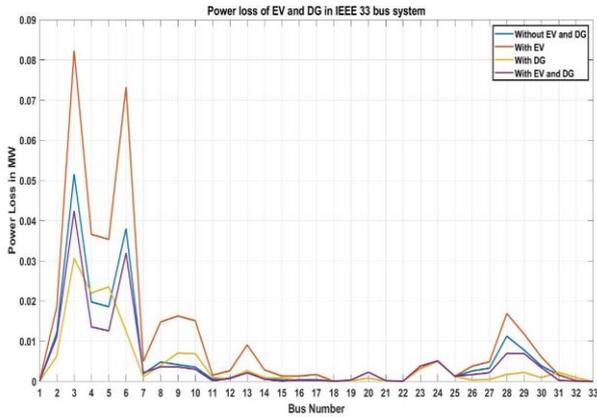
**Fig.7.** Power Losses in IEEE 33 Bus system with possible cases.
