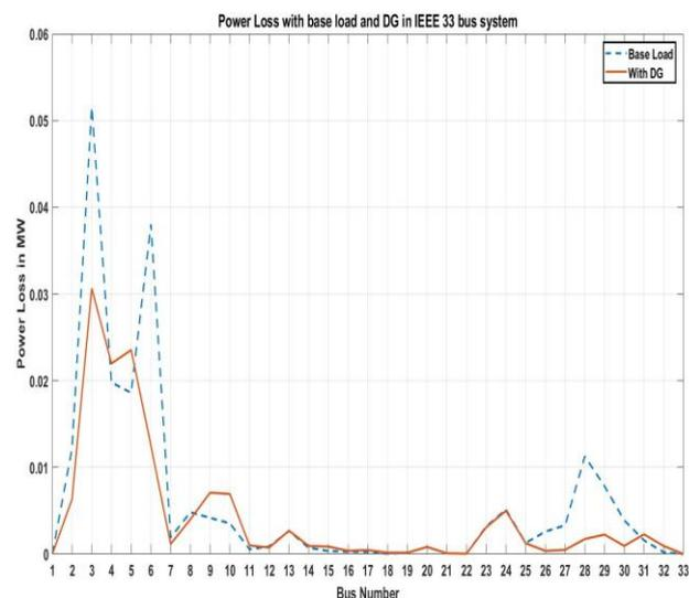
**Fig.2.** Power Loss of integrated DGs in distribution system.
