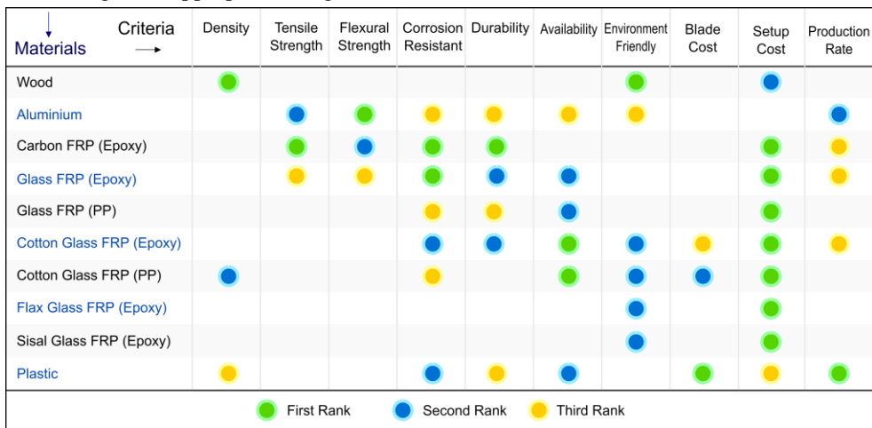
Fig. 3. The major three ranking criteria for considering alternative materials for SWT blades
