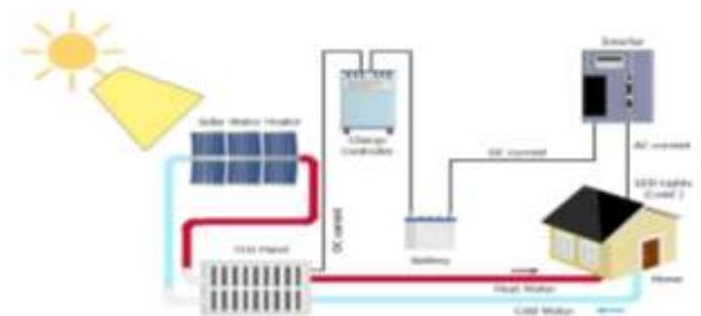
Figure 2. Role of TEG panel with solar water heater as renewable energy system.
