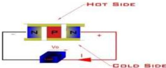
Fig. 1. Schematic diagram illustrating a TEG module.
