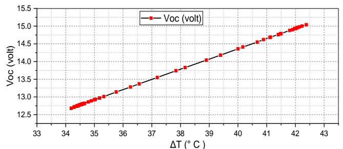
**Figure 7.** Open circuit voltage of the proposed 2 x 10 TEG panel.
