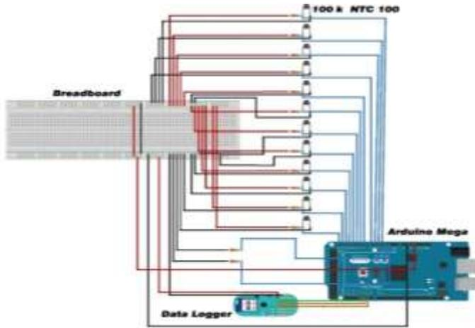
**Figure 5.** Temperature data logging via an Arduino Mega microcontroller.
