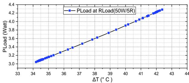
Figure 8. Load power of the proposed 2 x 10 TEG panel versus ΔT.
