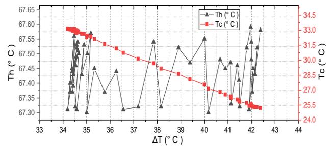
**Figure 6.**  $\Delta T$ ,  $T_h$  and  $T_c$  of a 2 x 10 TEG panel
