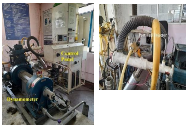
Fig. 3. Photograph of HCCI engine Experimental set-up
