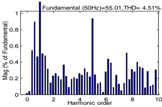
Fig. 5. 2. Source current THD with DC- DSTATCOM
