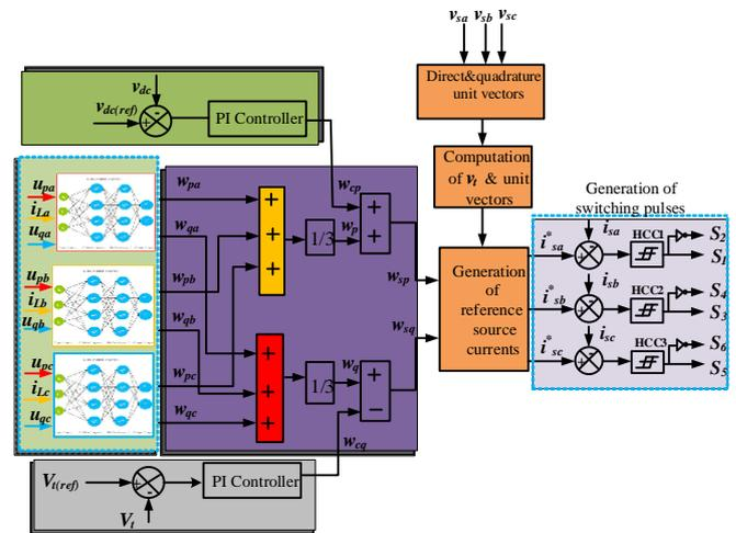
**Fig.5.**Block diagram of DBLN control technique
