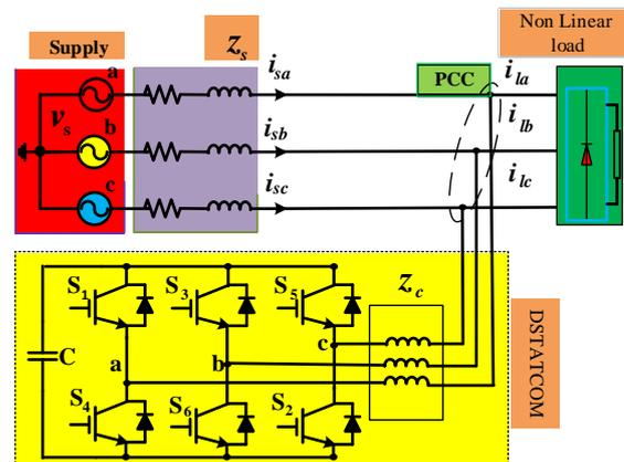
**Fig.3.** PDN with DC- DSTATCOM
