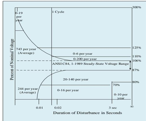
Fig.1. CBEMA curves for PDN faults versus voltage and duration
