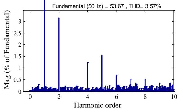
Fig.6.2. Source current THD with IC-DSTATCOM
