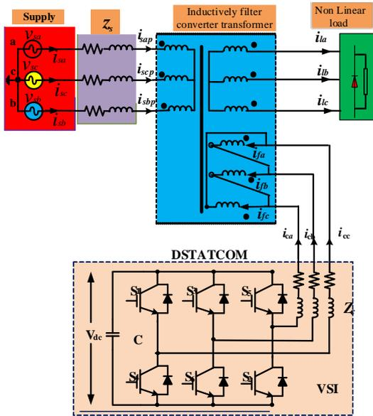
**Fig.4.** PDN with IC- DSTATCOM
