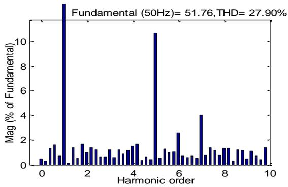
Fig. 5. 3. Load current THD with DC- DSTATCOM
