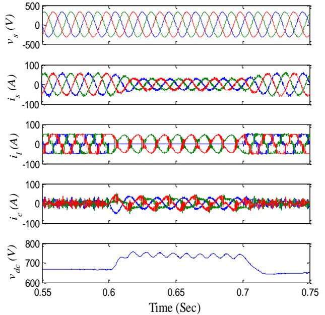
**Fig. 5.1** Results shown from (lower part of the waveform to upper); Inverter DC-link voltage, 3-phase compensating current, 3-phase non-linear load currents, 3-phase source currents and stable 3-phase supply voltage
