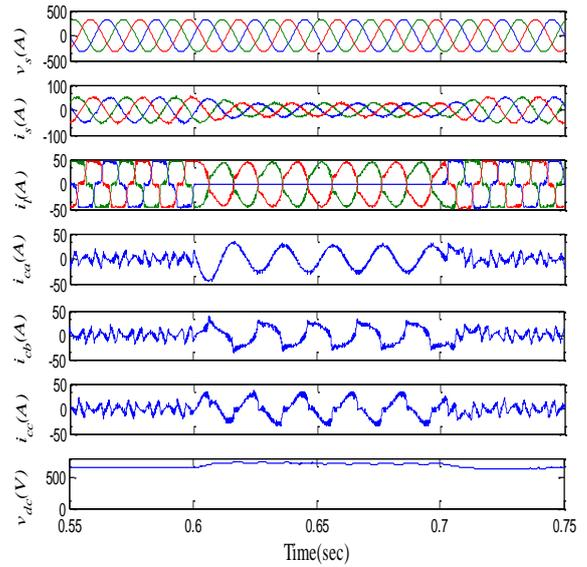
Fig.6.1. Results shown from (lower part of the waveform to upper); Inverter DC-link voltage, 3-phase compensating current, 3-phase non-linear load currents, 3-phase source currents and stable 3-phase supply voltage
