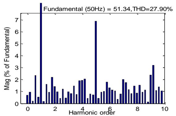
Fig.6. 3 Load current THD with IC-DSTATCOM
