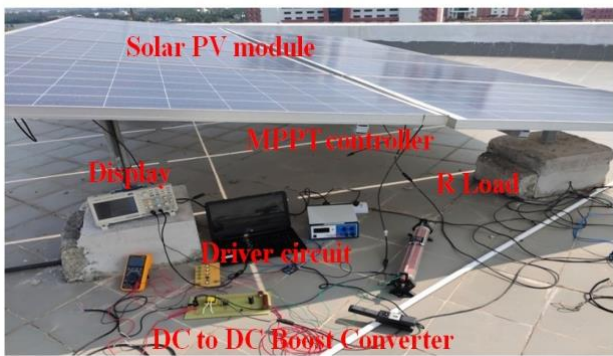
Fig.11 Hardware setup for the proposed MPPT scheme
