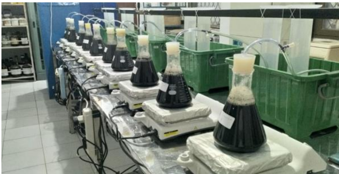
Fig. 2. Digester arrangement to evaluate onggok addition and delaying time in biogas production using tapioca wastewater.
