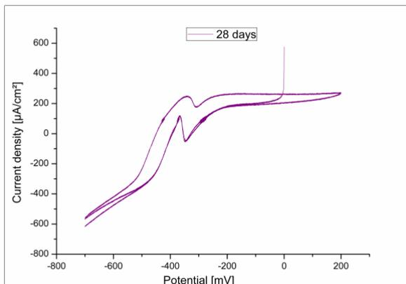
**Fig. 6.** CVs after 3 hours of polarisation at -0.2 V vs SCE of electrodes (open circuit time = 28 days) with scanning speed of 1 mV/s.
