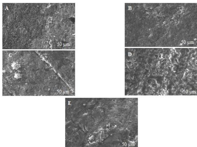
**Fig. 8.** Scanning electron microscopy of biofilms obtained after 3 hours polarization of biofilms: A control, B 8 days, C 14 days, D 28 days, E 35 days.
