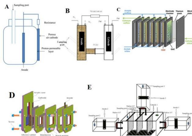
**Fig. 1.** Different microbial fuel cell designs: A) Single-chamber MFC [12], B) dual chamber [13], C) stacked MFC (SMFC) [14], D) plugged type soil microbial fuel cell (PSMFC) [15], E) multiple anode chamber and single cathode chamber microbial fuel cell (MAC-MFC) [16].
