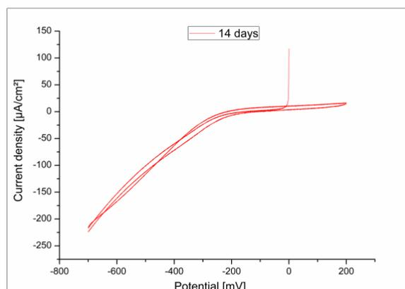
**Fig. 5.** CVs after 3 hours of polarisation at -0.2 V vs SCE of electrode (open circuit time = 14 days) with scanning speed of 1 mV/s.
