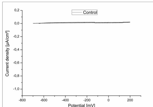
**Fig. 3.** CVs after 3 hours of polarisation at  $-0.2 V$  vs SCE of initial electrode with scanning speed of  $1 mV/s$ .
