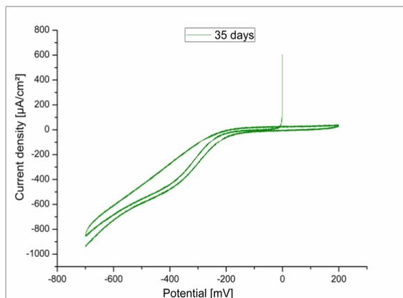
**Fig. 7.** CVs after 3 hours of polarisation at -0.2 V vs SCE of electrodes (open circuit time = 35 days) with scanning speed of 1 mV/s.
