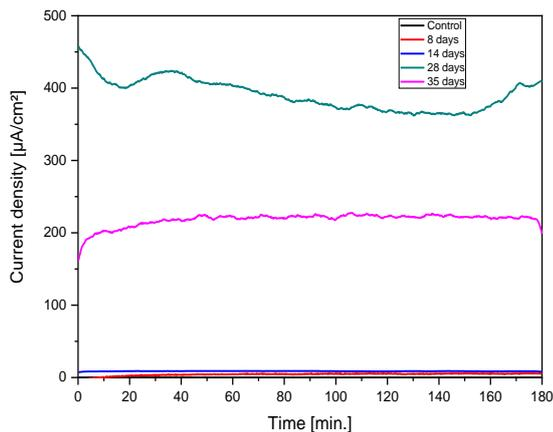
**Fig. 2.** Current densities ( $j$ ) obtained during 3h of polarization at  $-0.2V$  on biofilms at 8, 14, 28 and 35 days.
