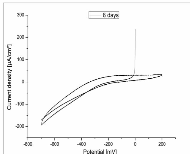
**Fig. 4.** CVs after 3 hours of polarisation at  $-0.2 V$  vs SCE of electrode (open circuit time = 8 days) with scanning speed of  $1 mV/s$ .
