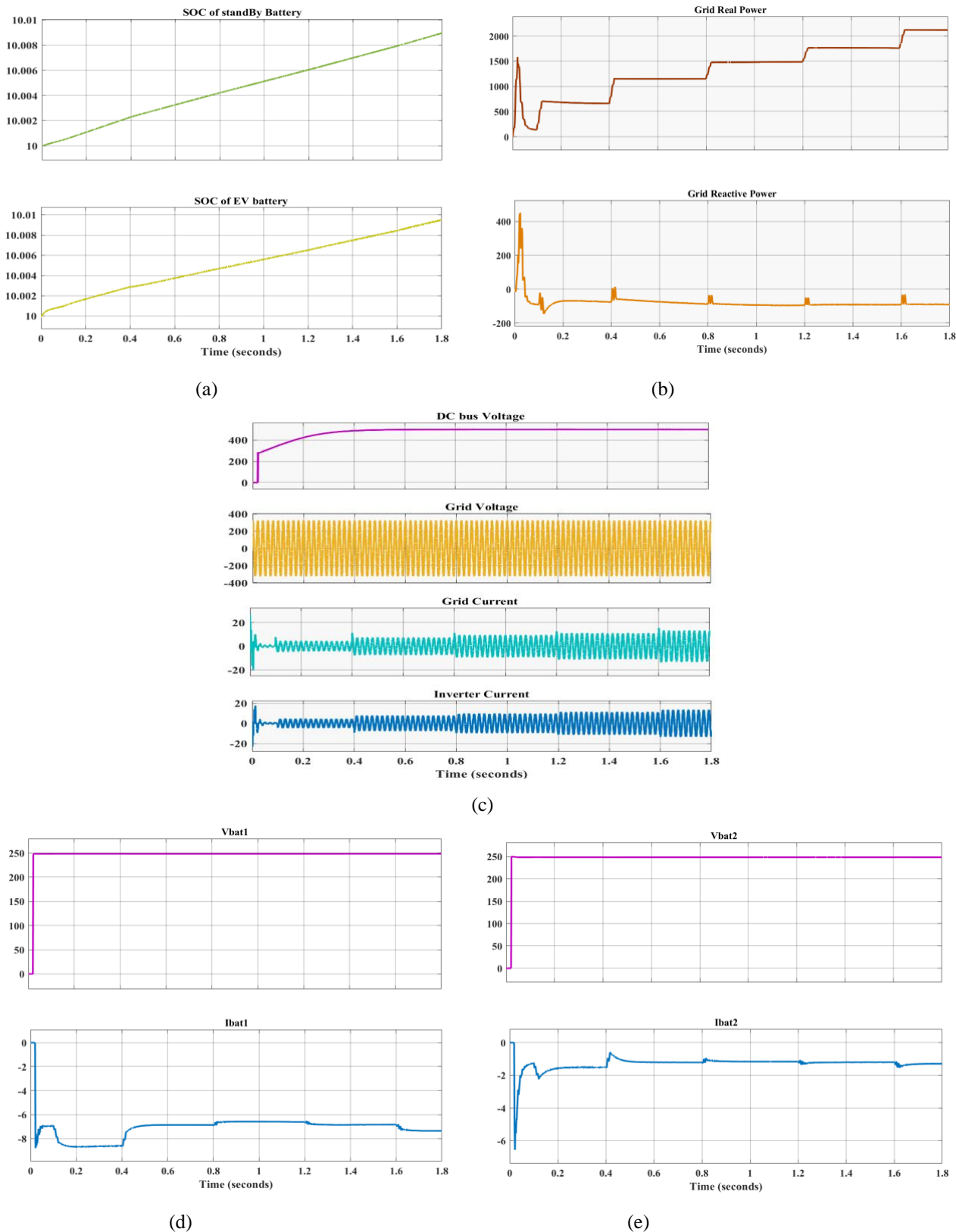
Fig. 11. Case with EV for PV Stationary Battery SOC_{bat} = 10\% (a) SOC of standby PV battery and EV battery (b) Grid real and reactive power (c) Grid side parameters (d) Standby PV battery parameters (e) EV battery charging parameters
