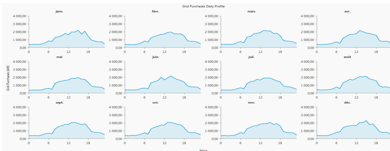
Fig. 12b. Rate of electric energy supplied by the network of photovoltaic system.
