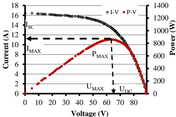
**Fig. 4.** The I-V and PV curves of the PV array ( $P_{G0}=1.6\text{KWp}$ ) at  $900\text{ W/m}^2$  of solar irradiance and the cell temperature is  $53^\circ\text{C}$ , 11/20/2014.
