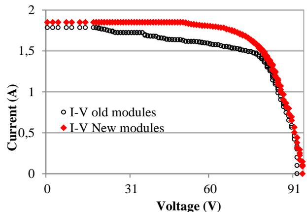
**Fig. 7.** The I-V curves of new and old PV modules at  $800\text{W/m}^2$  and cell temperature  $27^\circ\text{C}$ , 12/01/2014.
