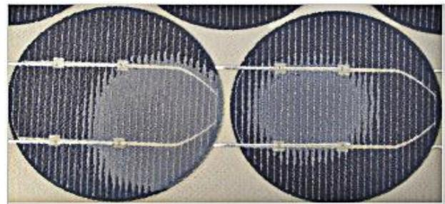
**Fig. 5.** The view of the delamination.
