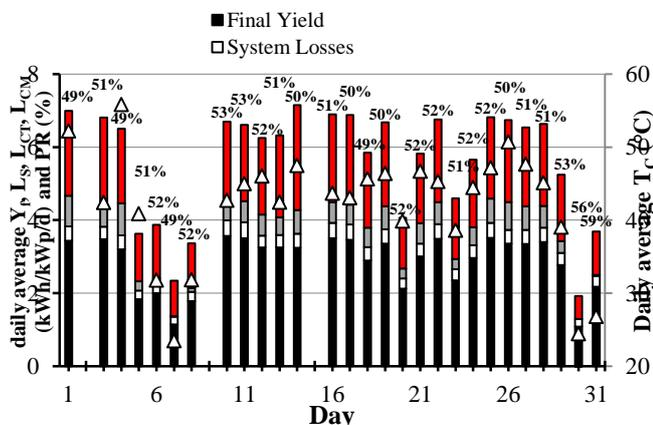
**Fig. 10.** The normalized daily final yield, system losses, thermal capture losses, miscellaneous capture losses and
