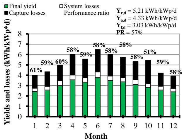
Fig. 9. Monthly daily average values of the Performance ratio, capture losses and system losses for 1.6kWp grid connected PV system at Batna region during the year 2013.
