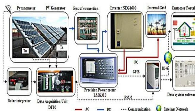
Fig. 2. Architecture of the smart home system installed at Batna University
