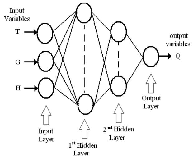
**Figure 9:** Schematic diagram of the construction of the adopted neural network model
