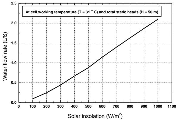
**Figure 6:** Variation of the Water flow rate of PVWPS with solar insolation at constant temperature and head.
