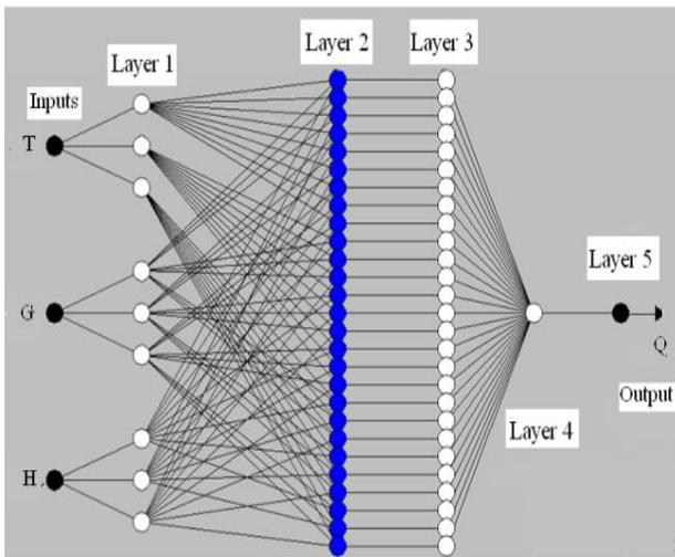
Figure 10: Schematic diagram of the adopted ANFIS model
