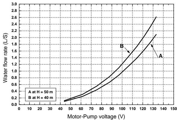
(b) The flow rate-voltage characteristics
