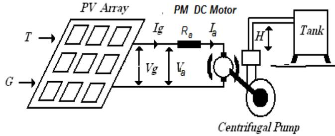
**Figure 1:** The proposed Photo-Voltaic Water Pumping System.
