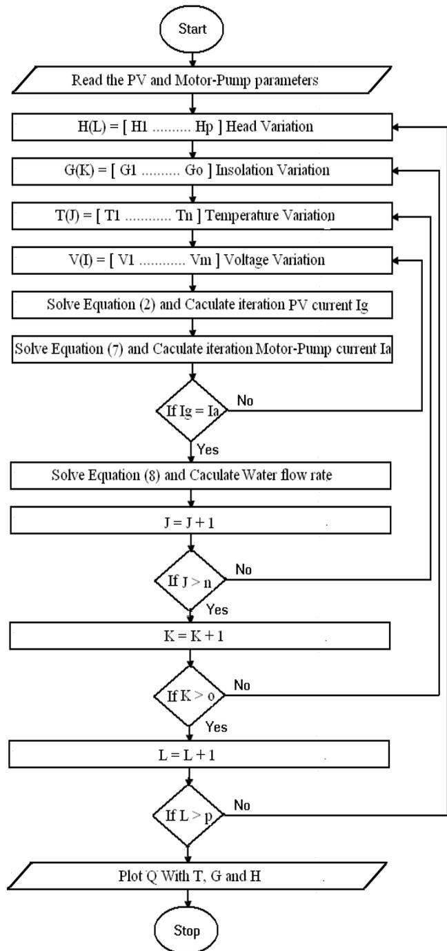
**Figure 5:** Procedure of PVWPS performance analysis using iteration technique
