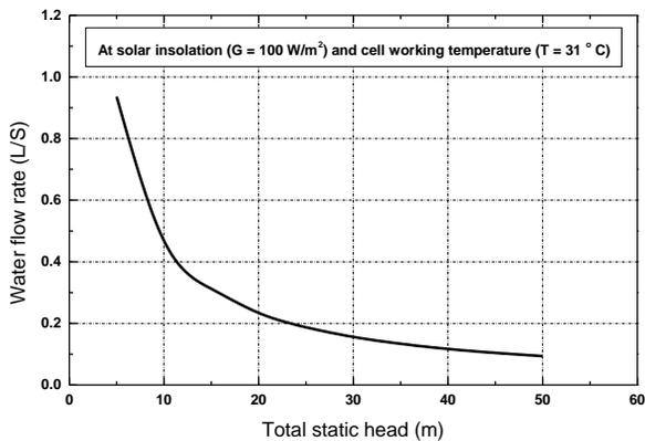
**Figure 8:** Variation of the Water flow rate of PVWPS with total static heads at constant insolation and temperature.
