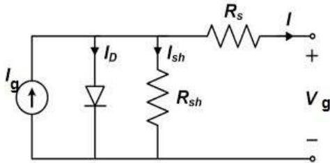
**Figure 2:** Equivalent electrical circuit of PV cell
