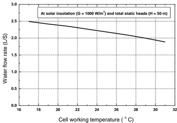
**Figure 7:** Variation of the Water flow rate of PVWPS with cell working temperature at constant insolation and head.
