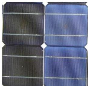
**Fig.16.** Defects in anti-reflecting coating in some modules
