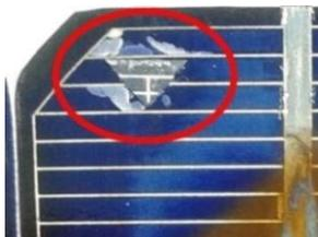
**Fig.15c** Cracks, lines and blemishes in some modules
