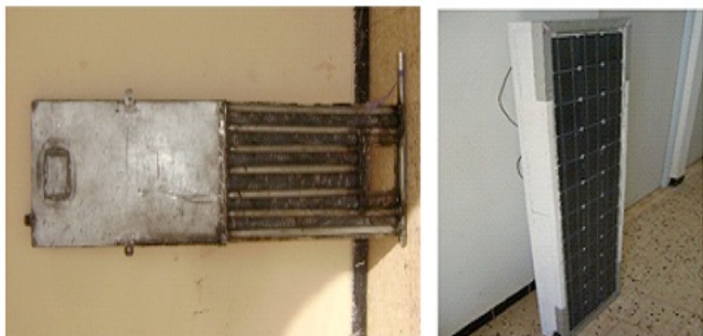
Fig. 3. Photo of the new PVT collector
