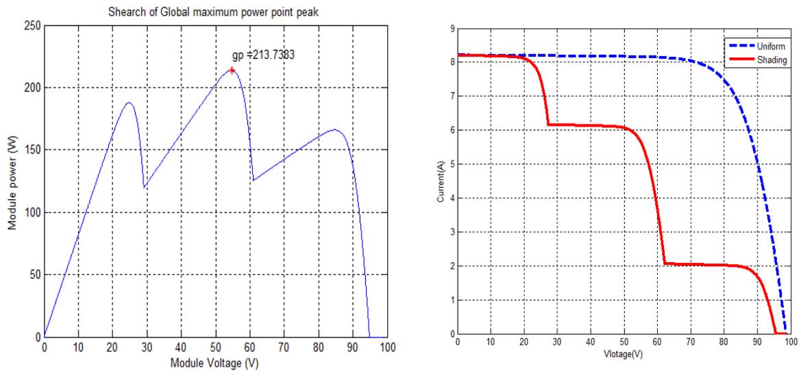
Fig.5. The resulting simulation of power-voltage and current-voltage curves.
