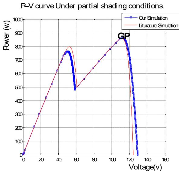
**Fig.11.** Simulation results of P–V curve at shading conditions.
