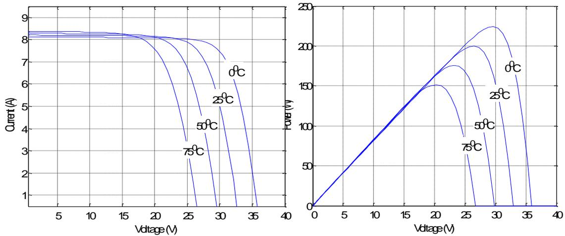
Fig.2. I-V and P-V characteristics under diverse temperatures.
