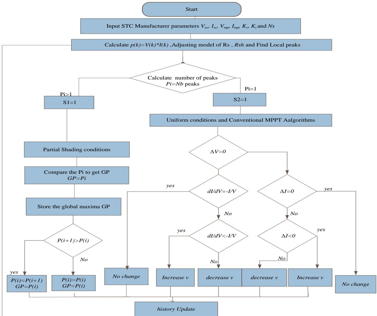
Fig.6. Flowchart for the GMPPT algorithm.
