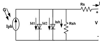
Fig.1. The circuit model of a photovoltaic cell.
