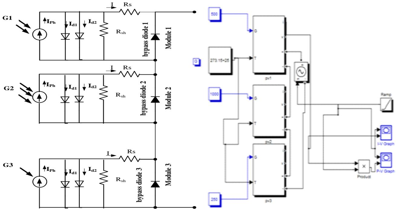
Fig.4. Simulation of 3 serial PV panels under partial shading conditions with bypass diodes using Matlab / Simulink.
