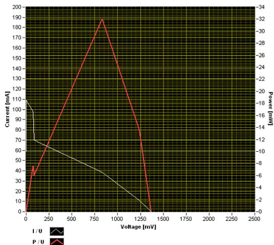
**Fig 8.** The I–V and P–V characteristic curves for the single stage Savonius turbine, at a 3 m/s wind speed
