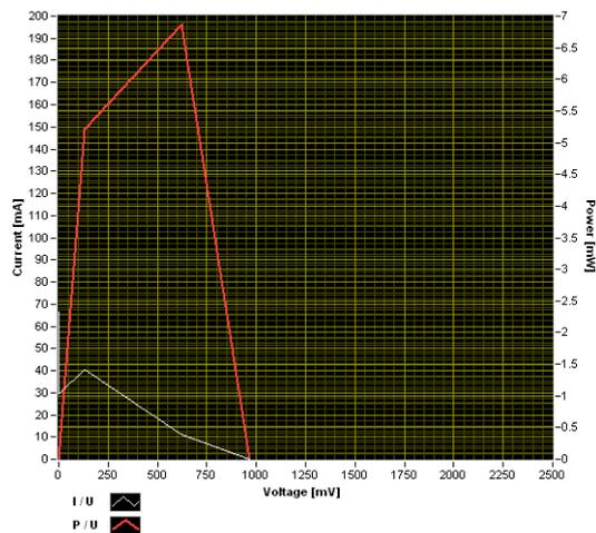
**Fig 10.** The I–V and P–V characteristic curves for type ‘Z’ Savonius turbine, at a 3 m/s wind speed
