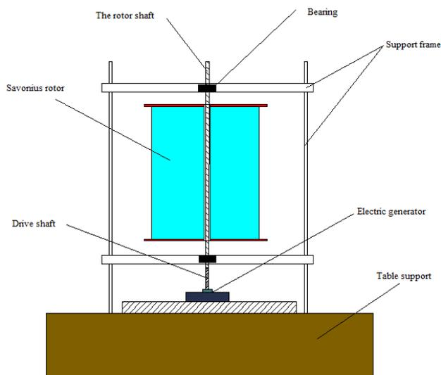
**Fig 6.** Savonius rotor connected directly at the electric generator
