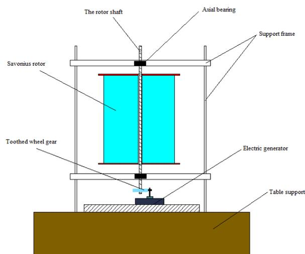
**Fig 7.** Savonius rotor connected to the generator through a toothed wheel gear
