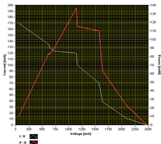
**Fig 15.** The I–V and P–V characteristic curves for the double stage Savonius turbine, at a 5 m/s wind speed
