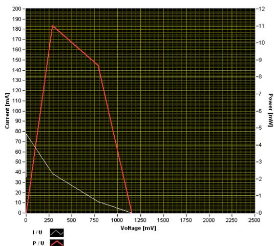
**Fig 9.** The I–V and P–V characteristic curves for the double stage Savonius turbine, at a 3 m/s wind speed
