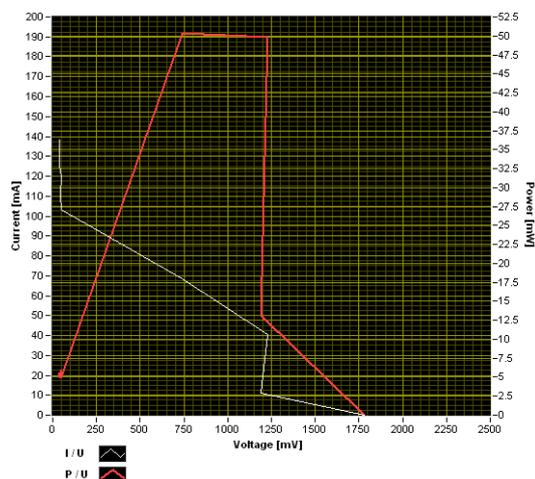
**Fig 11.** The I–V and P–V characteristic curves for the single stage Savonius turbine, at a 4 m/s wind speed
