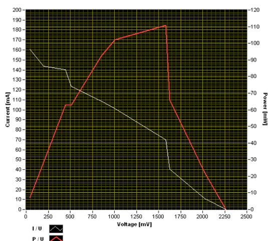
**Fig 14.** The I–V and P–V characteristic curves for the single stage Savonius turbine, at a 5 m/s wind speed
