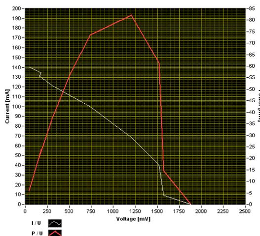
**Fig 16.** The I–V and P–V characteristic curves for type ,Z’ Savonius turbine, at a 5 m/s wind speed
