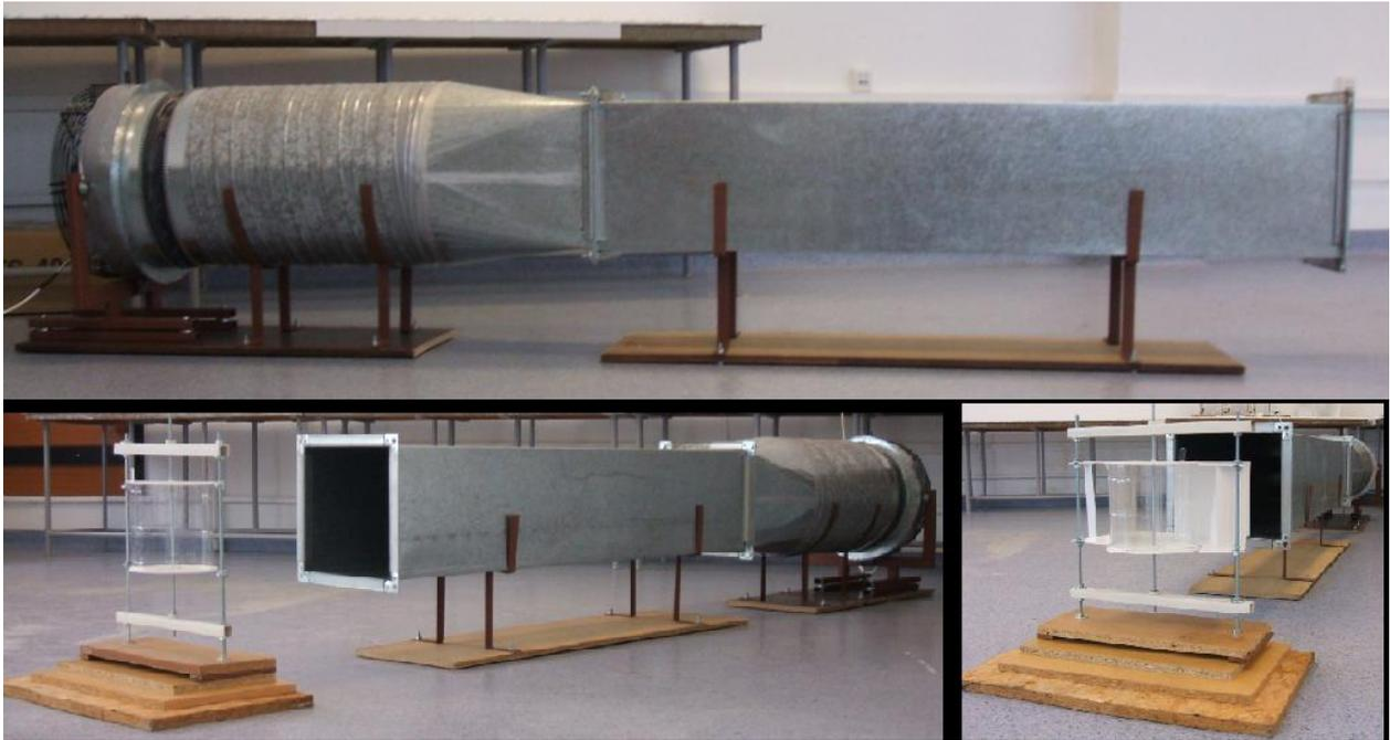
Fig 4. Open-circuit subsonic wind tunnel
