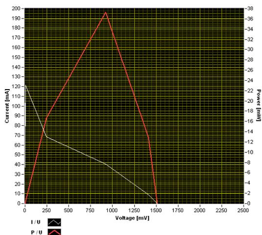
**Fig 13.** The I–V and P–V characteristic curves for type ,Z’ Savonius turbine, at a 4 m/s wind speed
