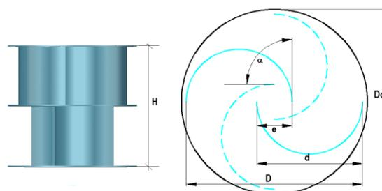
**Fig 2.** Double stage Savonius wind rotor
