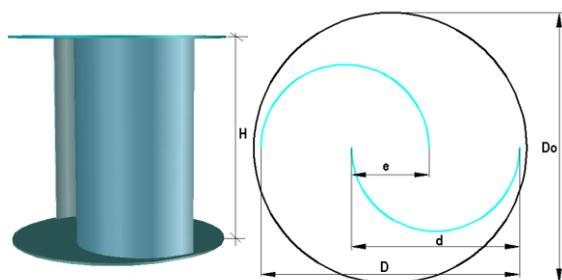
**Fig 1.** Single stage Savonius wind rotor
