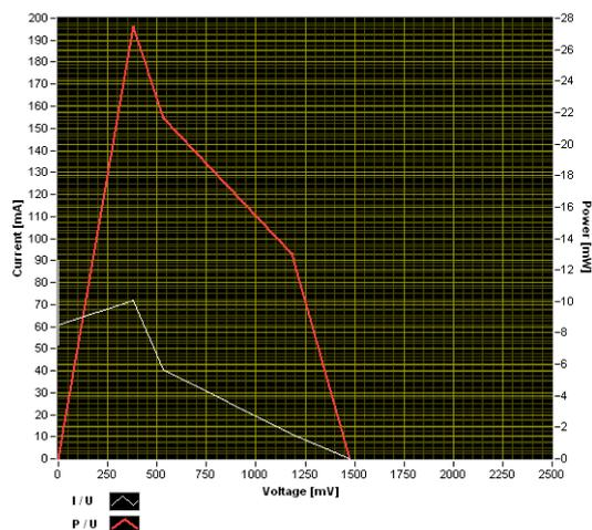
**Fig 12.** The I–V and P–V characteristic curves for the double stage Savonius turbine, at a 4 m/s wind speed
