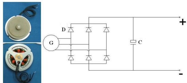
Fig 5. The schematic diagram of the CMC-30 generator
