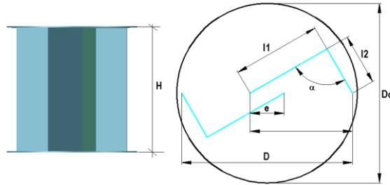
Fig 3. Type 'Z' Savonius wind rotor
