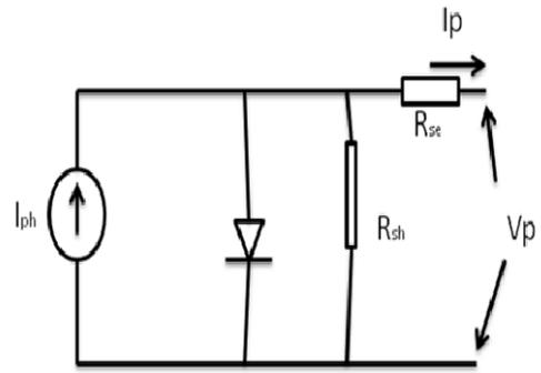
**Fig. 3** Solar Cell unit equivalent Circuit.
