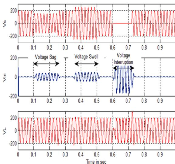
Fig. 12 Source, Injected & Load Voltages of ZSI-DVR model with ANFIS controller
