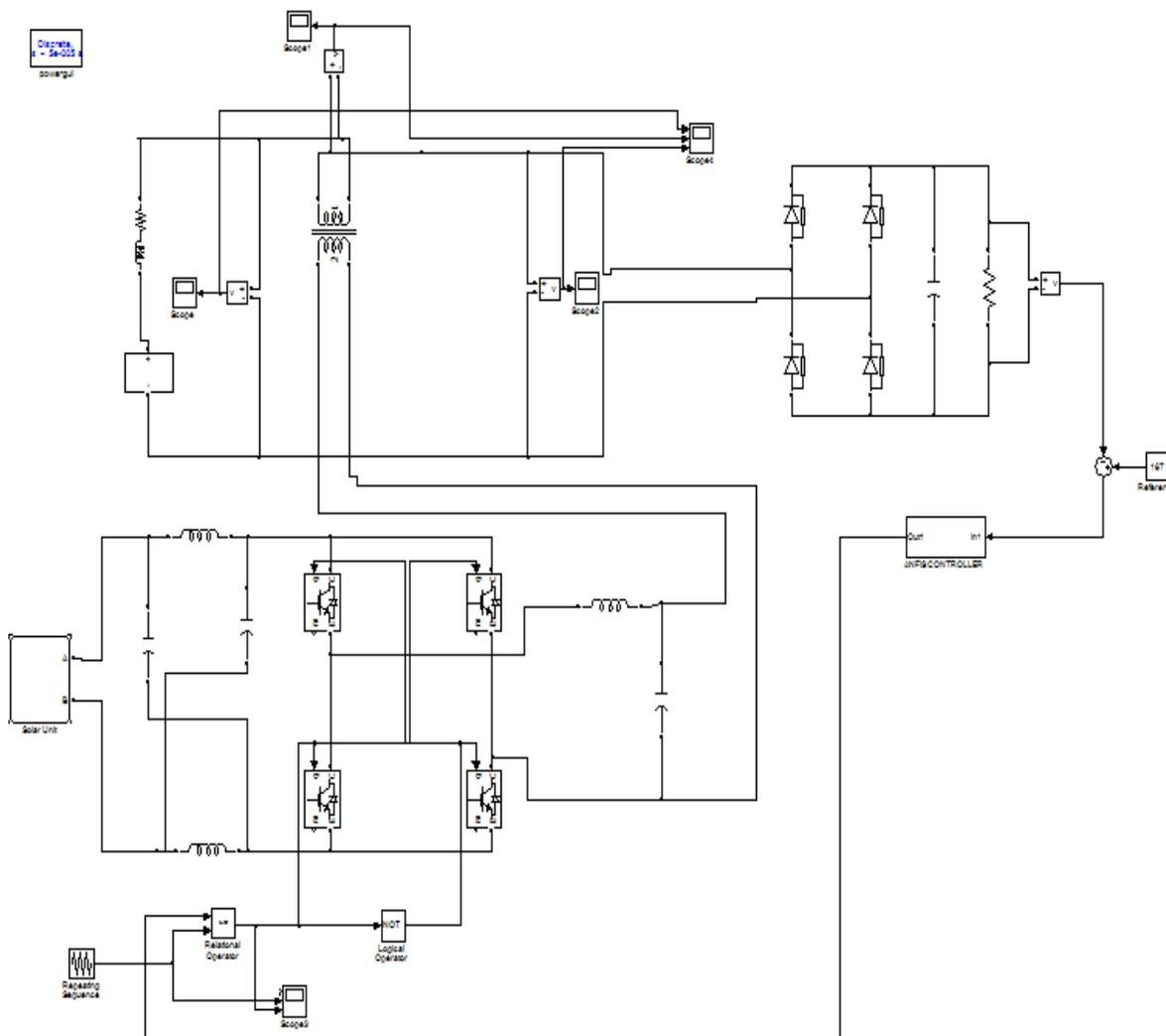
Fig 8a. Simulink Model of Proposed Dynamic Voltage Restorer for Voltage Disturbance Mitigation
