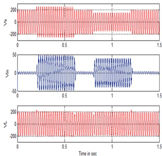
**Fig.9**Source, Injected & Load Voltages of PV ZSI-DVR with PI Controller
