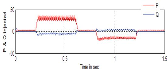
Fig. 11 Real and Reactive power injected by PV-ZSI-DVR
