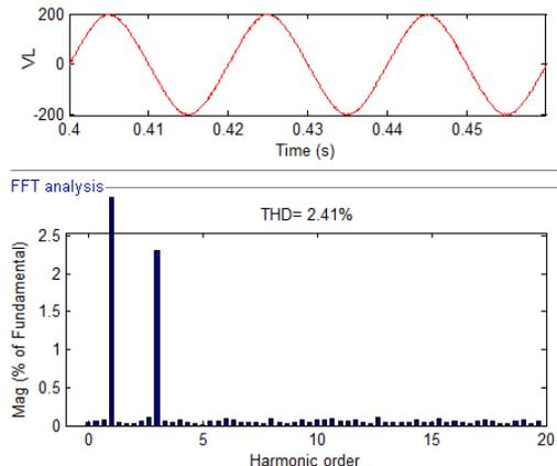
Fig.13%THD of Load Voltage is 2.41%
