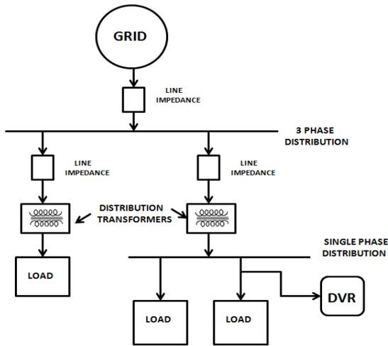
**Fig. 1** Block Diagram of DVR connected to Single Phase Distribution System.
