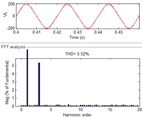
Fig. 10 %THD of Load Voltage is 5.52%
