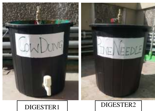
Fig.1. Pictorial view of DIGESTER1 & DIGESTER 2
