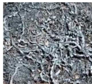
Fig. 2. The appearance of the steel chips after annealing and oxidation process
