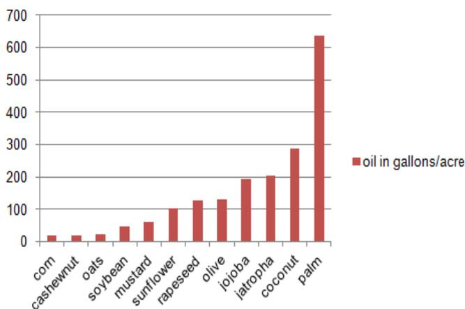
**Fig.1.** The quantity of oil obtained from different types of crops
