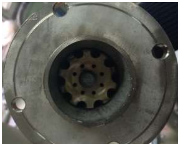
Fig. 2. The photograph of the existing natural gas burner
