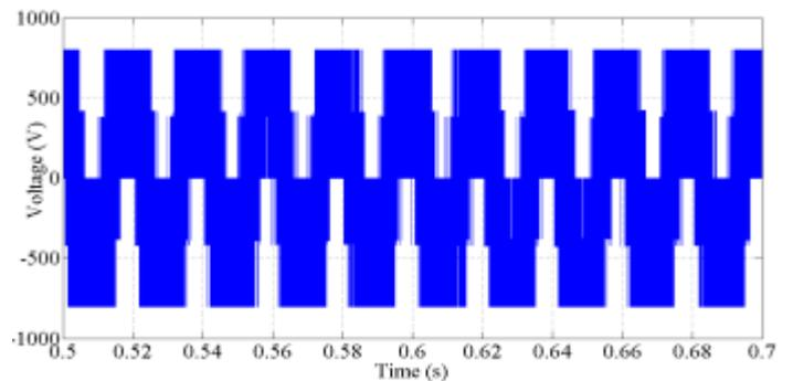
**Fig. 15** Output Voltage of TLI based STATCOM
