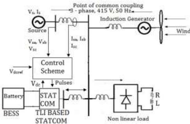
**Fig.2** Grid connected system with control scheme
