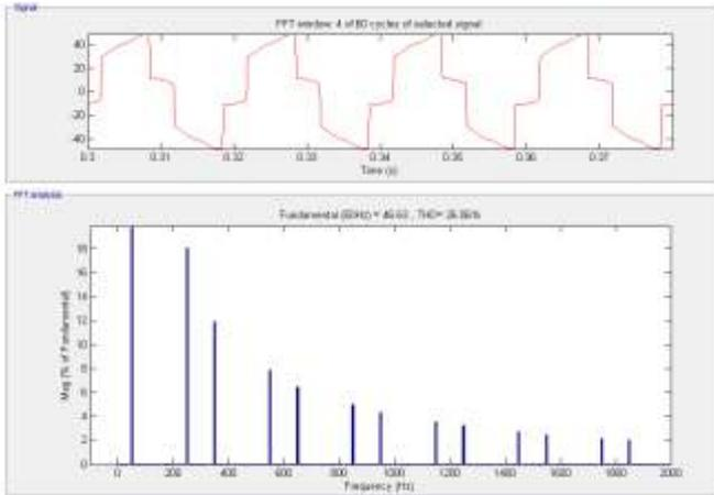
Fig. 6 FFT analysis of Source current waveform without STATCOM
