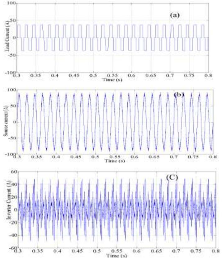
Fig. 8 (a) Load Current (b) Source Current (c) Inverter Injected Current, for CTLI based STATCOM with HCC
