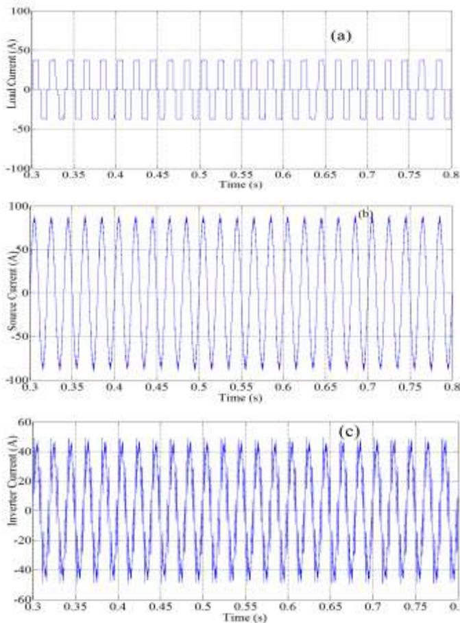
**Fig. 12** (a) Load Current (b) Source Current (c) Inverter Injected Current, for the TLI based STATCOM with HCC
