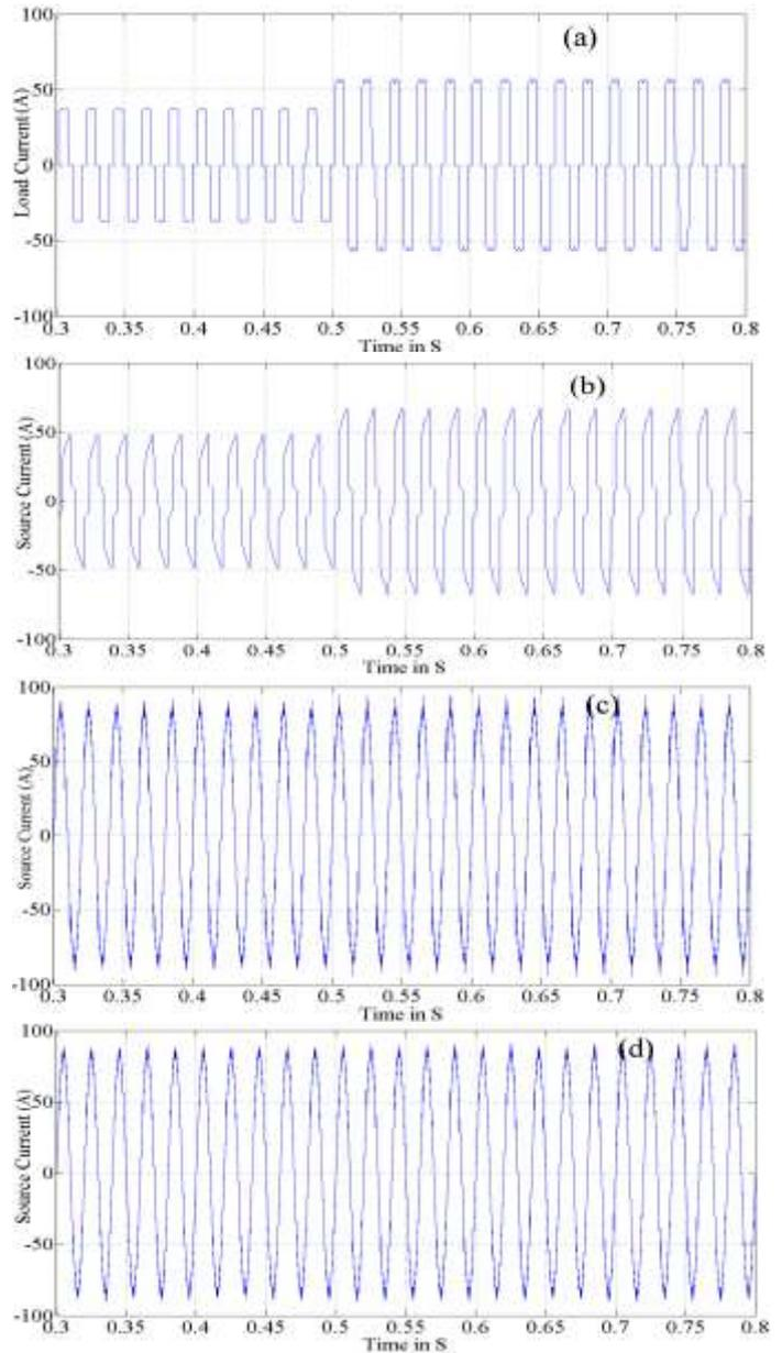
**Fig. 17** (a) Load current (b) source current without STATCOM (c) Source current with CTLI based STATCOM (d) Source current with TLI based STATCOM during dynamic load changes
