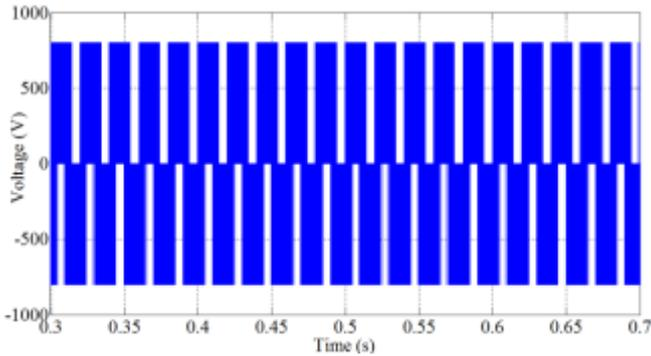
**Fig. 11** Output Voltage of CTLI based STATCOM
