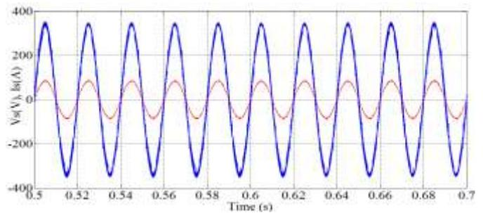
**Fig. 14** Supply voltage & supply current at PCC with the TLI based STATCOM with HCC
