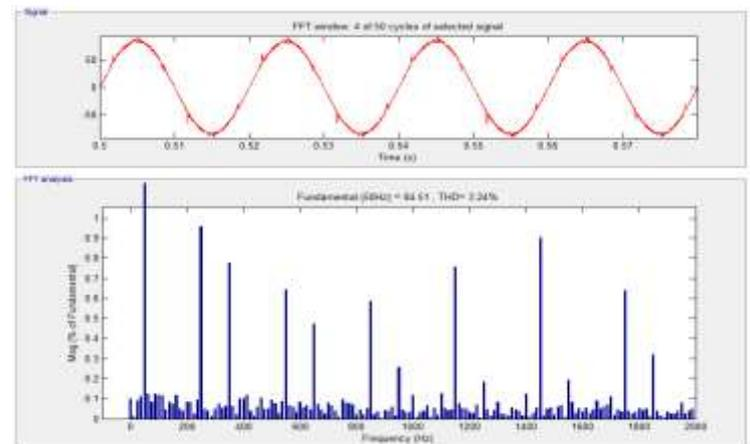
Fig. 9 FFT analysis of Source current waveform with CTLI based STATCOM with HCC
