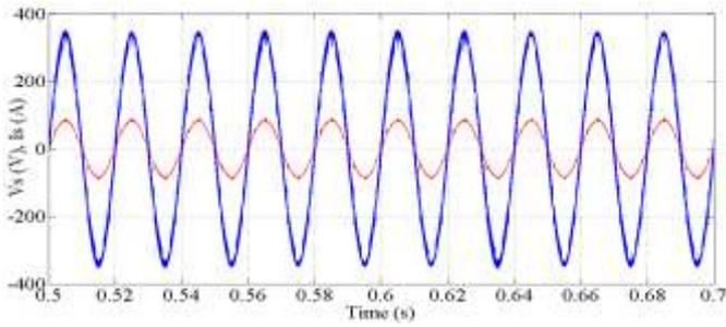
**Fig. 10** Supply voltage & supply current at PCC with CTLI based STATCOM with HCC
