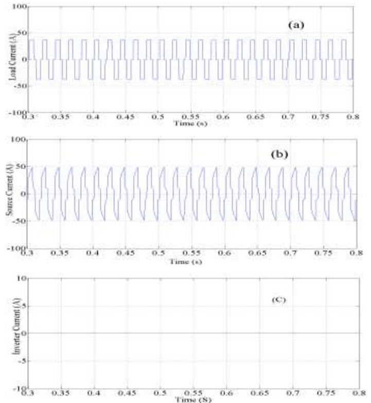
Fig.5 (a) Load Current (b) Source Current (c) Inverter Injected Current, Without STATCOM
