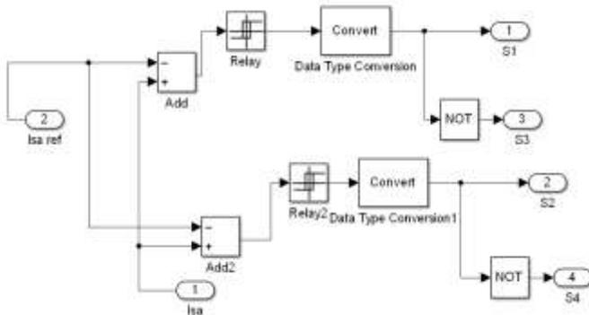
Fig. 4 Switching signals generation for phase A
