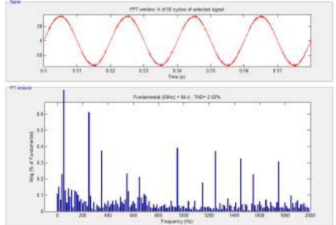
**Fig. 13** FFT analysis of Source current waveform of TLI based STATCOM with HCC
