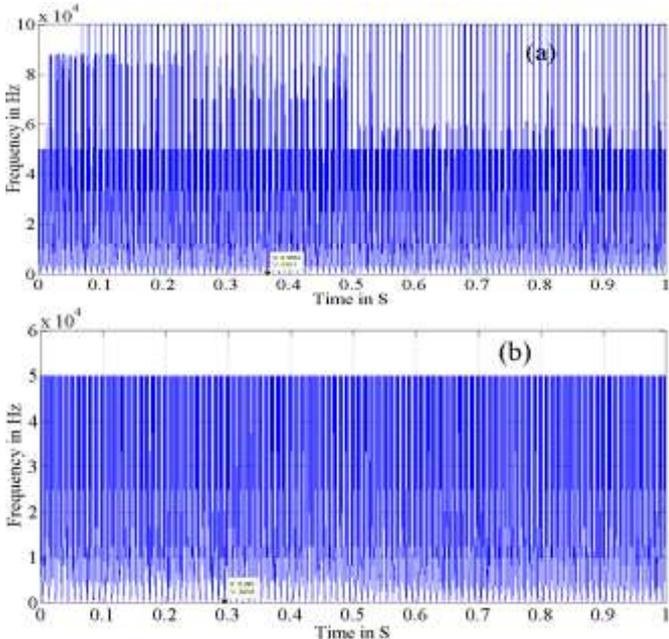
**Fig. 16** Switching frequency (a) CTLI based STATCOM (b) TLI based STATCOM
