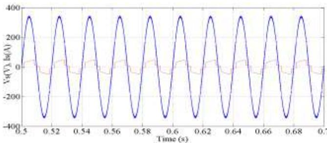
Fig. 7 Supply voltage & supply current at PCC without STATCOM
