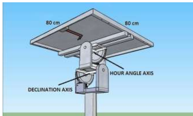
Fig. 2. Mechanical structure for the dual-axis solar tracker.
