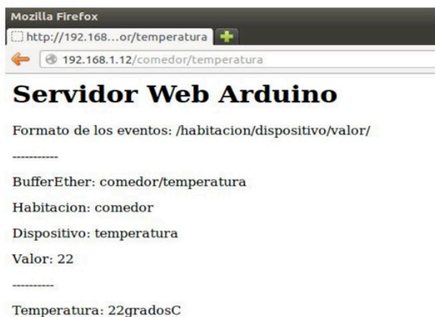
Figure 1. Web server based on Arduino [3].
