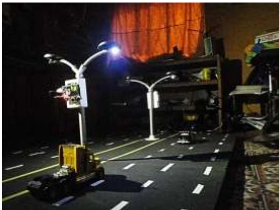
Figure 11: Luminaires lit with vehicular flux [15]
