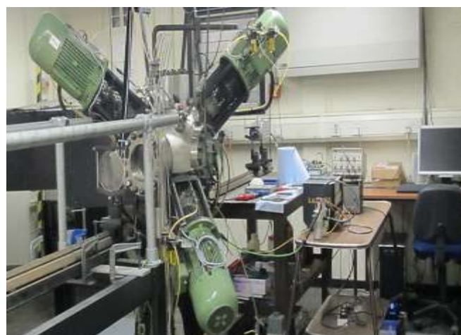
Fig. 1. Mk2 spherical combustion bomb system with spark ignition in the centre of the bomb
