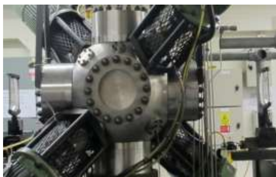
Fig. 3. 380mm diameter of Mk2 spherical bomb
